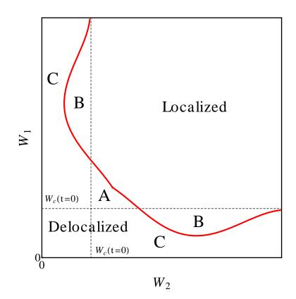
Figure 5.4: Schematic phase diagram for the coupled Bethe lattices with identical hopping but different disorder obtained from the results in Figs. 5.2 and 5.3. The red curve separates the  $W_1 - W_2$  plane to the localized and delocalized regimes. For a guide to the eye we indicate the critical disorder for the uncoupled lattices  $W_c(t=0) \approx 17.3$  by the bashed lines.
