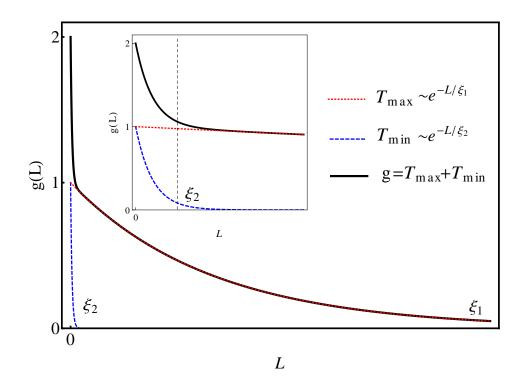
Figure 4.3: Schematic diagram for typical values of dimensionless conductance g as a function of the length L in the case  $\xi_1 \gg \xi_2$ . A crossover happens at  $L \sim \xi_2$ . In the region  $L < \xi_2$ , g decays as fast as  $T_{\min}$  (see the insert). Once  $L > \xi_2$ , g decays as slowly as  $T_{\max}$ . The system is well conducting if  $L < \xi_1$  and crosses to an insulating regime for  $L > \xi_1$ .
