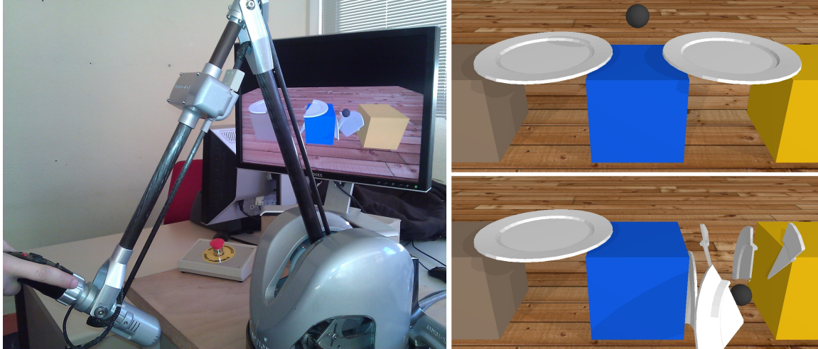
Figure 5.8 – Setup of the experiment. Left : photography of the experimental conditions. The haptic interface is linked to the ball in the simulation, and the user can break the plates with force feedback. Right : screenshots of the simulation during a trial at the initial condition (top) and after one plate has been broken (right).
