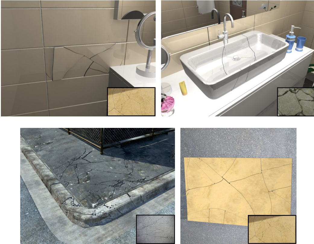
Figure 5.5 – Application of our example-based fracturing method on different scenes. Photographs of input fracture patterns are shown in the insets. Left to right: (1) a bathroom tile has been broken, and each fragment can be manipulated separately. (2) Fracture pattern obtained from a ground tile photograph applied on a basin. (3) Sidewalk and curb from an urban scene fractured
