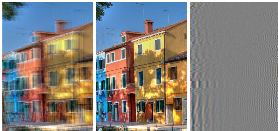
Figure A.17 – Rand code : observed image (left). The blur interval length is equal to 52 pixels here. Reconstructed image ( RMSE = 2.01 ) (middle). Residual noise (difference between ground truth and reconstructed, dynamic normalized on [0, 255] by an affine contrast change).
