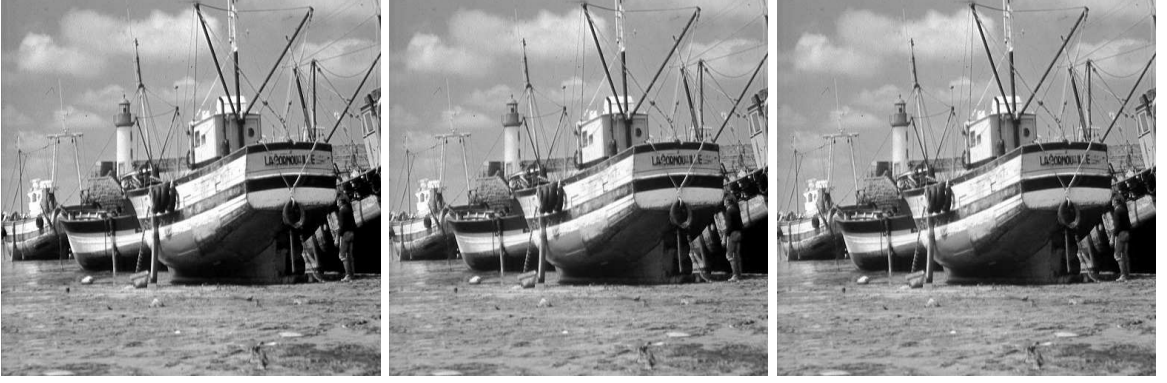
Figure A.3 – On the left : an uncorrupted test image (boat). On the middle : the result of the MIRE algorithm ( s^* = 0 ); the produced image is the same. This experiment was done using [132]. On the right : the result of the locally adaptive variant of MIRE described in section 5.1 ( s^* = 0 everywhere in the image). As predicted the algorithm does not make the image worse or create artifacts (safety check). Results on real raw images corrupted with non uniformity are detailed in section 6.
