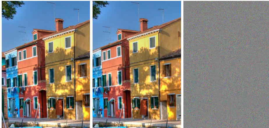
Figure A.19 – Sinc code : observed image (left). The blur interval length is equal to 52 pixels here. Reconstructed image ( RMSE = 1.33 ) (middle). Residual noise (difference between ground truth and reconstructed, dynamic normalized on [0, 255] by an affine contrast change). The acquired image is “sharp”, it is no surprise since the sinc-code has a nearly constant Fourier transform thus, it does not alter any frequency.
