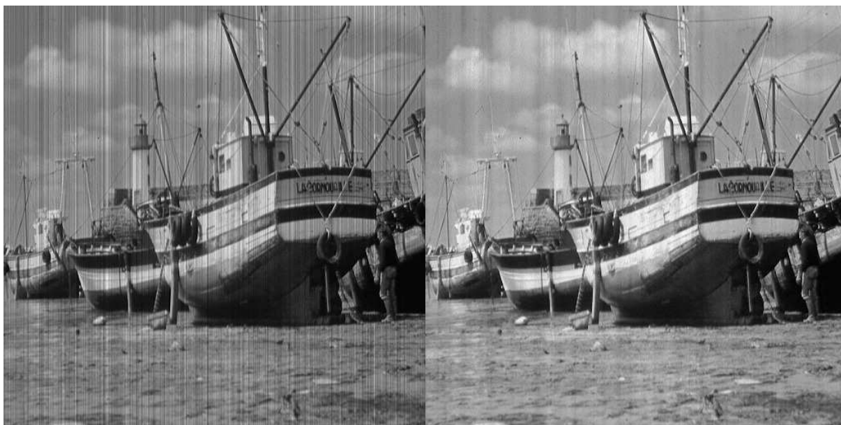
Figure A.6 – On the left : an image with a strong simulated non linear non uniformity . On the right : the image processed by the proposed algorithm. RMSE = 9.6629 , RMSE^{CI} = 5.7314 .
