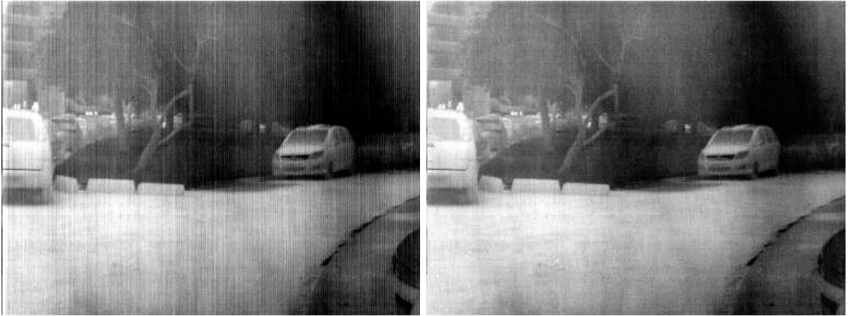
Figure A.10 – On the left : a real raw image taken by an infrared camera. On the right the result of ADMIRE.
