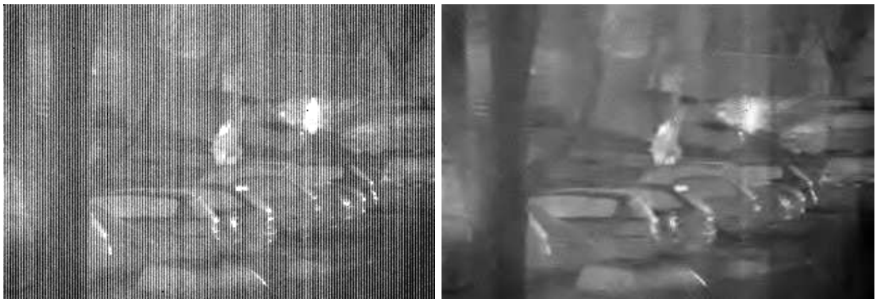
Figure A.15 – On the left : a real raw image taken by an infrared camera. On the right the result of ADMIRE.
