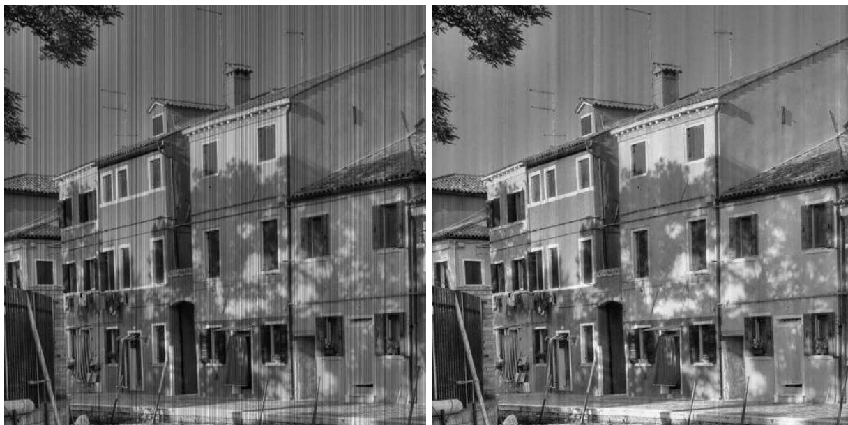
Figure A.7 – On the left : an image with a strong simulated non linear non uniformity . On the right : the image processed by the proposed algorithm. RMSE = 8.7100 , RMSE^{CI} = 7.3411 .
