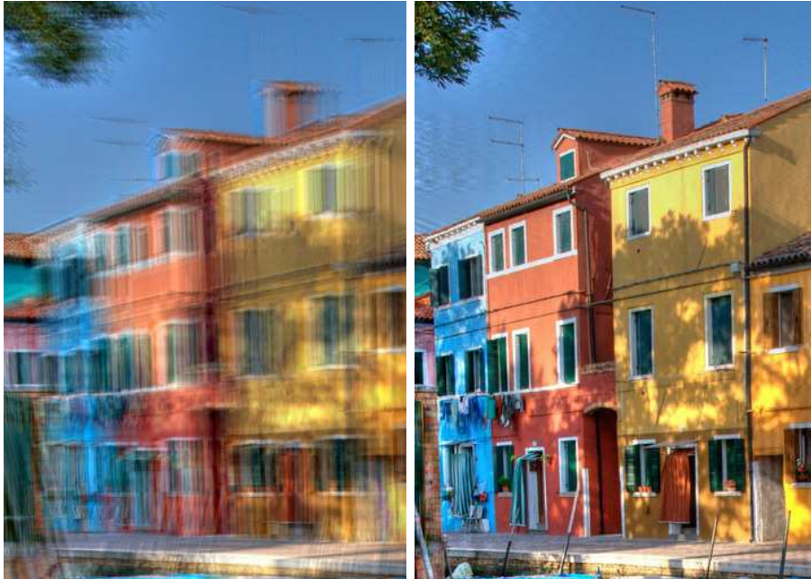
Figure 3 – Left: simulated noisy and blurry image acquired by a flutter shutter camera with a 52 pixels blur support. Right: restored image. Those images were generated from a flutter shutter camera simulator [128]. It simulates a flutter shutter camera assuming a Poisson photon emission. Such a deconvolution is not possible without a flutter shutter .
