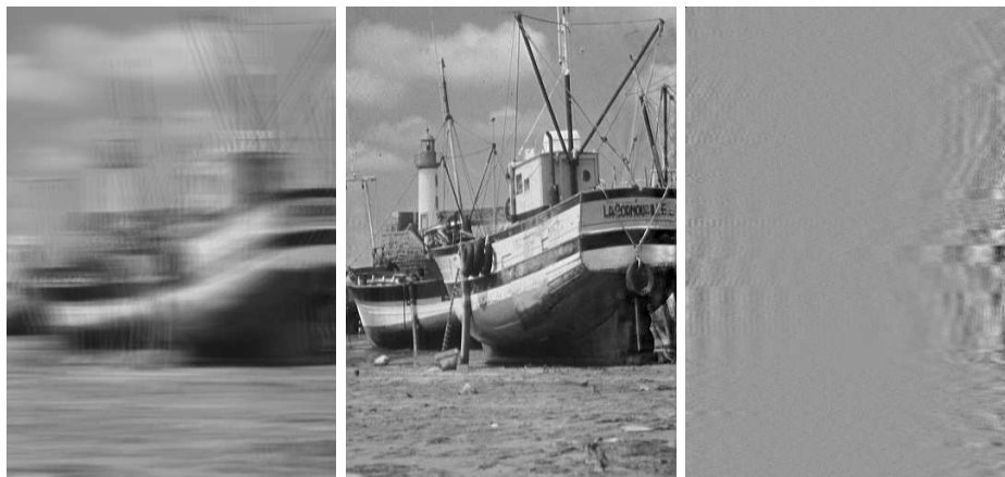
Figure A.10 – Agrawal et al. code : observed image (left). The blur interval length is equal to 52 pixels here. Reconstructed image ( RMSE = 2.54 ) (middle). Residual noise (difference between ground truth and reconstructed, dynamic normalized on [0, 255] by an affine contrast change).
