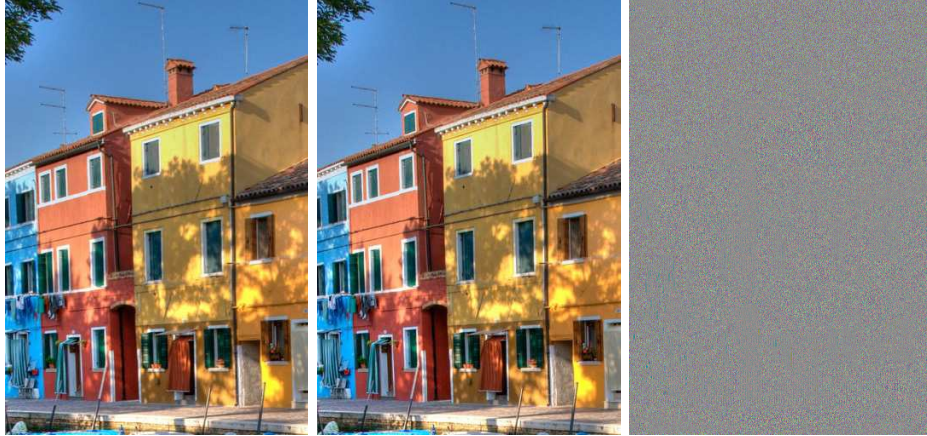
Figure A.14 – Snapshot : observed image (left). The blur interval length is equal to 1 pixel here. Reconstructed image ( RMSE = 1.34 ) (middle). Residual noise (difference between ground truth and reconstructed, dynamic normalized on [0, 255] by an affine contrast change).
