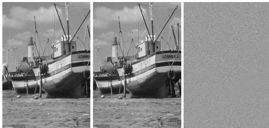
Figure A.13 – Sinc code : observed image (left). The blur interval length is equal to 52 pixels here. Reconstructed image ( RMSE = 1.46 ) (middle). Residual noise (difference between ground truth and reconstructed, dynamic normalized on [0, 255] by an affine contrast change). The acquired image is “sharp”, it is no surprise since the sinc-code has a nearly constant Fourier transform thus, it does not alter any frequency.
