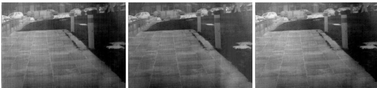
Figure A.9 – On the left : a real raw image of an outdoor scene taken by an infrared camera. Middle : the total variation based method. Notice the artifacts created below the poles. On the right the proposed method (we deactivate the DCT denoising to provide a fair comparison).
