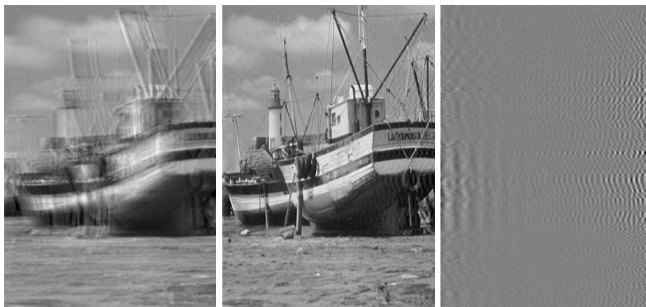
Figure A.11 – Rand code : observed image (left). The blur interval length is equal to 52 pixels here. Reconstructed image ( RMSE = 2.25 ) (middle). Residual noise (difference between ground truth and reconstructed, dynamic normalized on [0, 255] by an affine contrast change).
