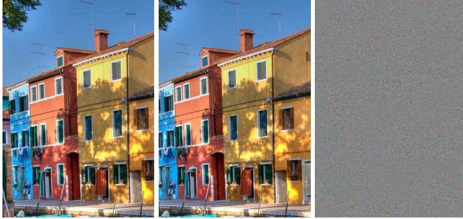
Figure A.2 – Sinc code : observed image (left). The blur interval length is equal to 52 pixels here. Reconstructed image ( RMSE = 1.33 ) (middle). Residual noise (difference between ground truth and reconstructed, dynamic normalized on [0, 255] by an affine contrast change). The acquired image is “sharp”, it is no surprise since the sinc -code has a nearly constant Fourier transform thus, it does not alter any frequency.
