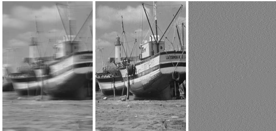
Figure A.12 – M.I.P. code : observed image (left). The blur interval length is equal to 52 pixels here. Reconstructed image ( RMSE = 2.31 ) (middle). Residual noise (difference between ground truth and reconstructed, dynamic normalized on [0, 255] by an affine contrast change).
