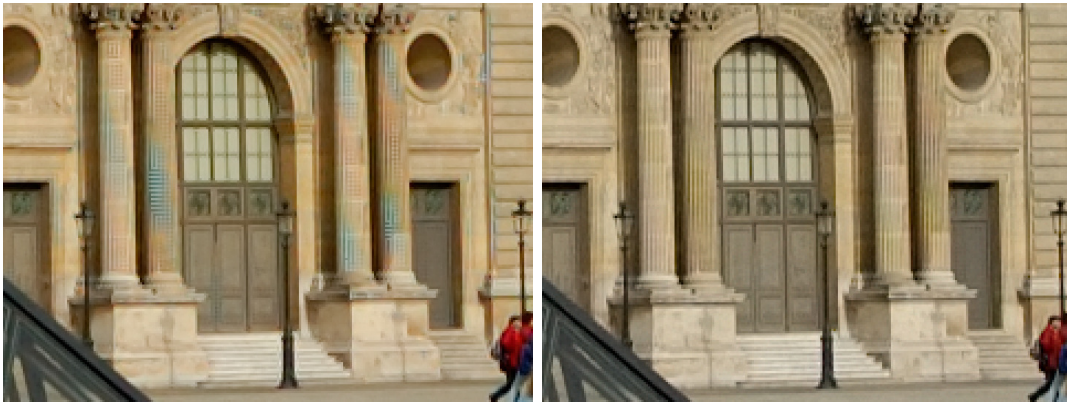
Figure 6.7: Wrong and good demosaicking: Nikon NX and Buades, Coll, Morel Algorithm (in DxO OPv5).
