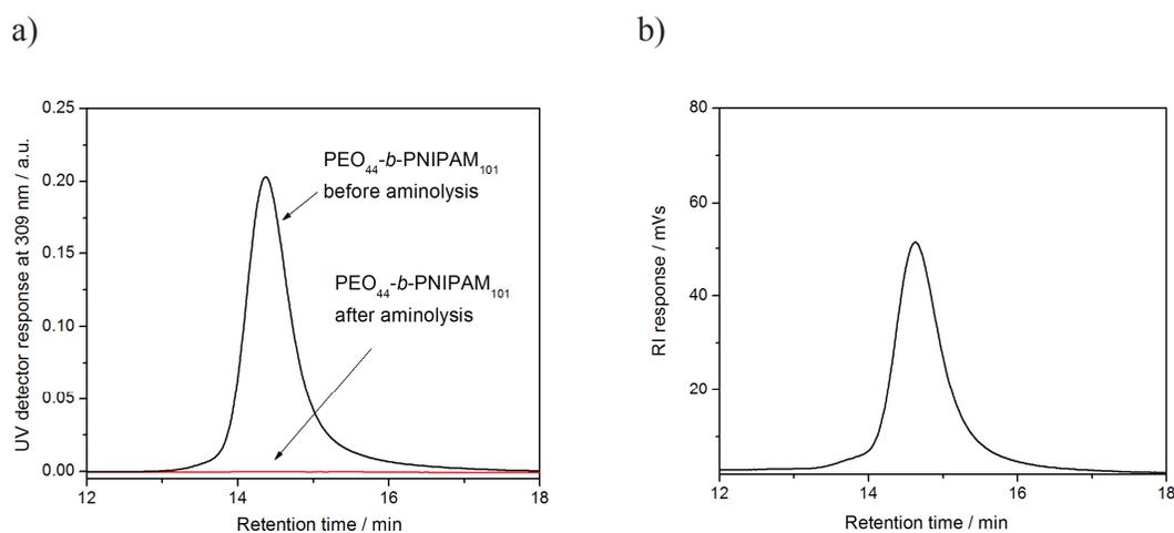
*Figure 8: a) Overlay of SEC traces of  $\text{PEO}_{44}\text{-}b\text{-PNIPAM}_{101}$  before and after aminolysis using UV detection at 309 nm and, b) SEC trace of  $\text{PEO}_{44}\text{-}b\text{-PNIPAM}_{101}$  after aminolysis using RI detection.*
