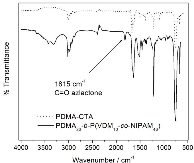
Figure 6: FT-IR spectrum for PDMA<sub>23</sub>-b-P(VDM<sub>10</sub>-co-NIPAM<sub>46</sub>) block copolymer compared with the FT-IR spectrum of PDMA-CTA.
