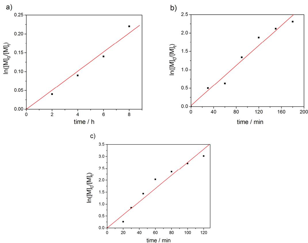
*Figure 4: Kinetic plots for the RAFT polymerizations of: a) styrene,  $[S]_0:[(3)]_0:[ACVA]_0 = 49:1:0.1$ , b) ethyl acrylate,  $[EA]_0:[(3)]_0:[ACVA]_0 = 50:1:0.1$  and c) N-isopropyl acrylamide,  $[NIPAM]_0:[(3)]_0:[ACVA]_0 = 55:1:0.1$ , using ACVA as the initiator and the azlactone-functionalized trithiocarbonate (3) as the RAFT agent in dioxane at 70°C.*
