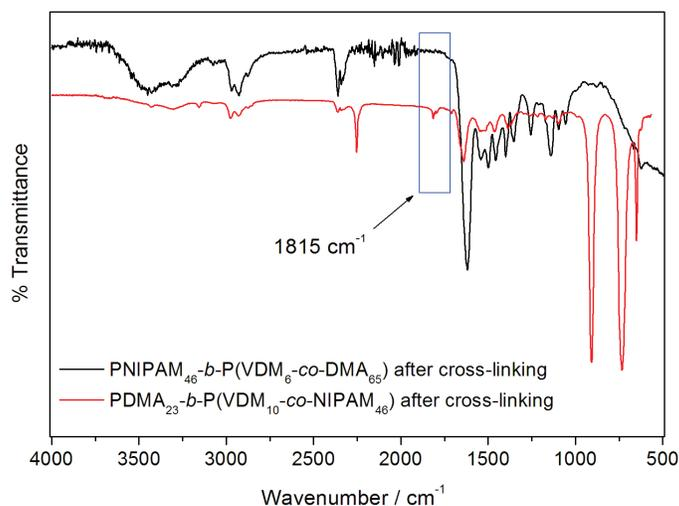
*Figure 9: Comparison of FT-IR spectra of the cross-linked nanoparticles issued from PNIPAM<sub>46</sub>-b-P(VDM<sub>6</sub>-co-DMA<sub>65</sub>) and PDMA<sub>23</sub>-b-P(VDM<sub>10</sub>-co-NIPAM<sub>46</sub>) block copolymers.*
