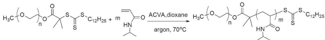
Scheme 4: RAFT polymerization of NIPAM using PEO-CTA as the macromolecular chain transfer agent and using ACVA as the initiator in dioxane at  $70^\circ\text{C}$ .
