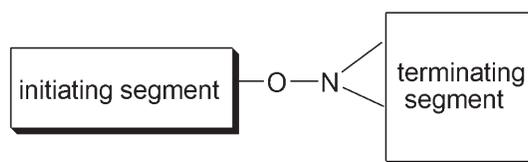
*Figure 1: General structure of an alkoxyamine.*
