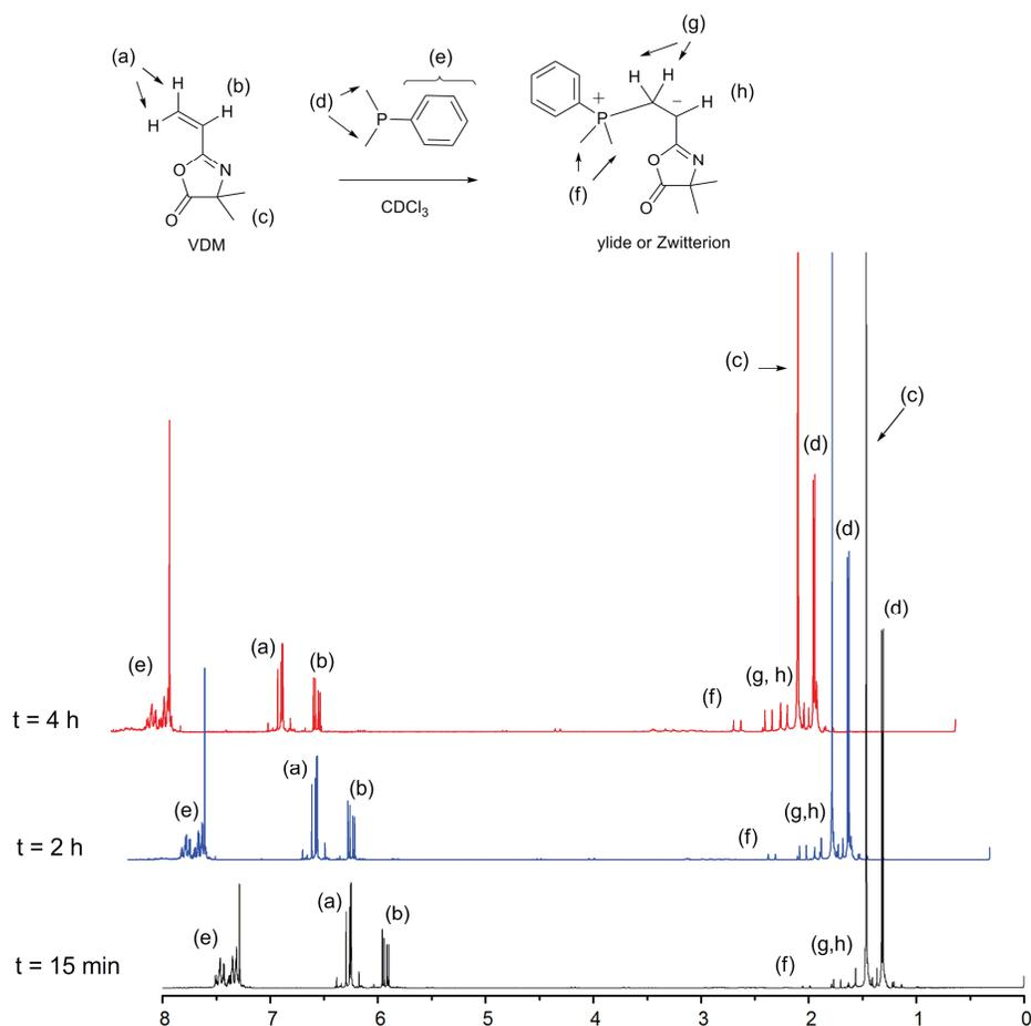
Figure 8: Online  $^1\text{H}$  NMR spectra at  $t = 15$  min,  $t = 1$  hour and  $t = 4$  hours for the reaction between DMPP and VDM in  $\text{CDCl}_3$  ( $[\text{VDM}]_0 : [\text{DMPP}]_0 = 1 : 1.2$ ).
