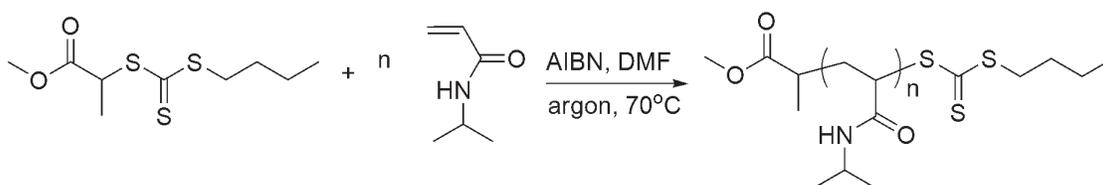
*Scheme 1: RAFT polymerization of NIPAM using MBTTCP as the RAFT agent and AIBN as the initiator in DMF at 70°C, [NIPAM]<sub>0</sub>: [MBTTCP]<sub>0</sub>: [AIBN]<sub>0</sub> = 24:1:0.2.*
