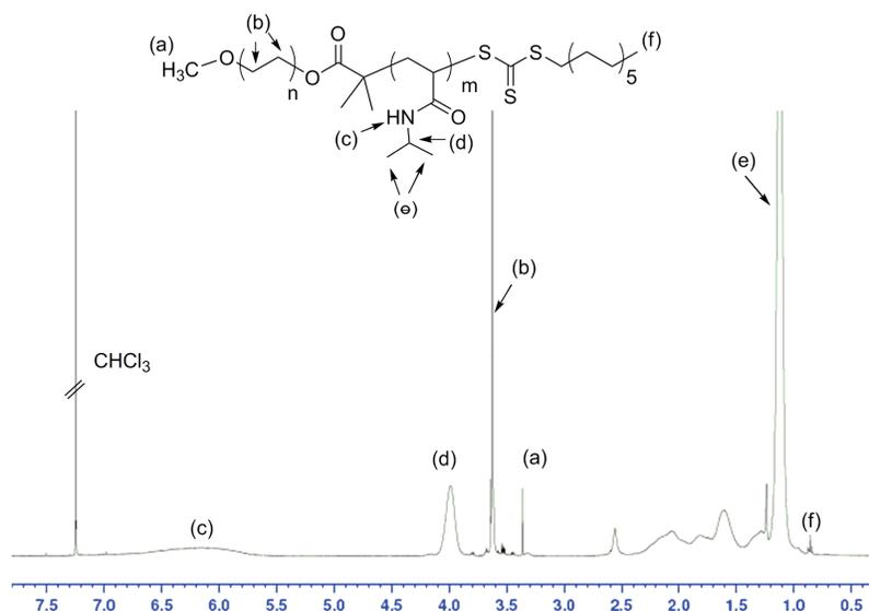
Figure 7:  $^1\text{H}$  NMR spectrum of  $\text{PEO}_{44}\text{-}b\text{-PNIPAM}_{101}$  in  $\text{CDCl}_3$ .
