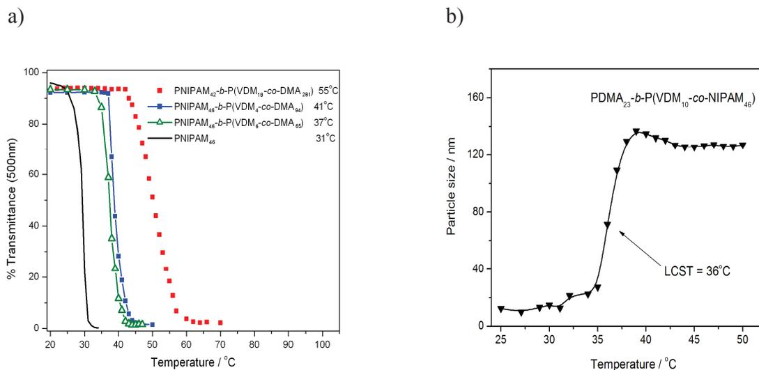
Figure 7: Measured LCST of block copolymers in aqueous solution: a) using UV-Vis spectrophotometry at 500 nm for PNIPAM-*b*-P(VDM-*co*-DMA) block copolymers, b) using DLS for PDMA-*b*-P(VDM-*co*-NIPAM) block copolymer.
