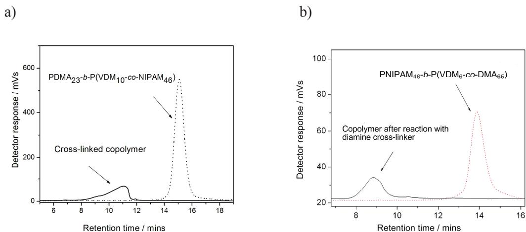
Figure 8: SEC traces of: a) the  $PDMA_{23}$ - $b$ - $P(VDM_{10}$ - $co$ - $NIPAM_{46})$  block copolymer prior to cross-linking and after cross-linking using 2,2'-ethylenedioxybis(ethylamine) and, b) the  $PNIPAM_{46}$ - $b$ - $P(VDM_6$ - $co$ - $DMA_{66})$  block copolymer prior to cross-linking and after cross-linking using 2,2'-ethylenedioxybis(ethylamine).
