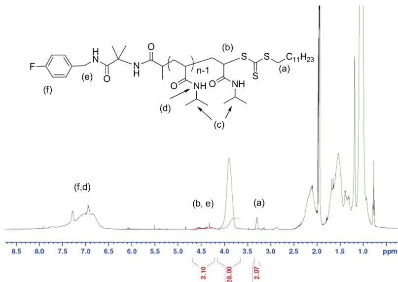
Figure 12:  $^1\text{H}$  NMR spectrum (solvent: acetone  $D_6$ ) of the polymer obtained after reacting the  $\alpha$ -azlactone- $\omega$ -dodecyltrithiocarbonate PNIPAM with 4-fluorobenzylamine at room temperature in THF for 24h.
