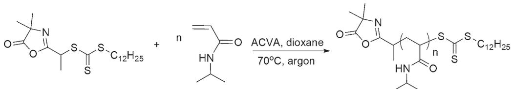
Scheme 10: RAFT polymerization of *N*-isopropyl acrylamide using  $[NIPAM]_0/[3]_0/[ACVA]_0 = 55/1/0.1$  in dioxane at 70°C.
