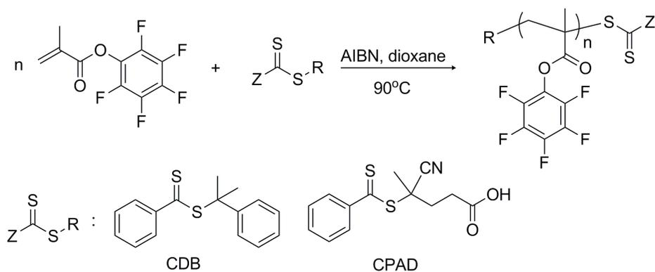
Scheme 61: Synthesis of PPFPMAs via RAFT polymerization.
