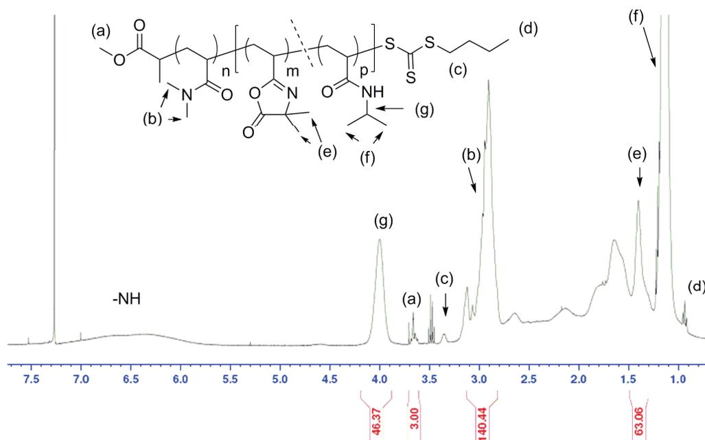
*Figure 4:*  $^1\text{H}$  NMR spectrum of the PDMA<sub>23</sub>-*b*-P(VDM<sub>10</sub>-*co*-NIPAM<sub>46</sub>) block copolymer in CDCl<sub>3</sub>.
