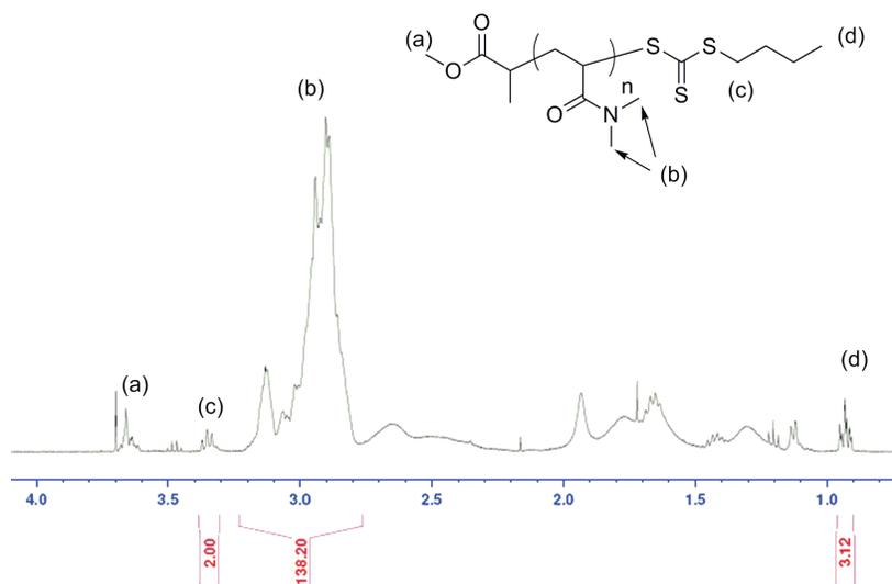
Figure 1:  $^1\text{H NMR}$  of PDMA in  $\text{CDCl}_3$ .
