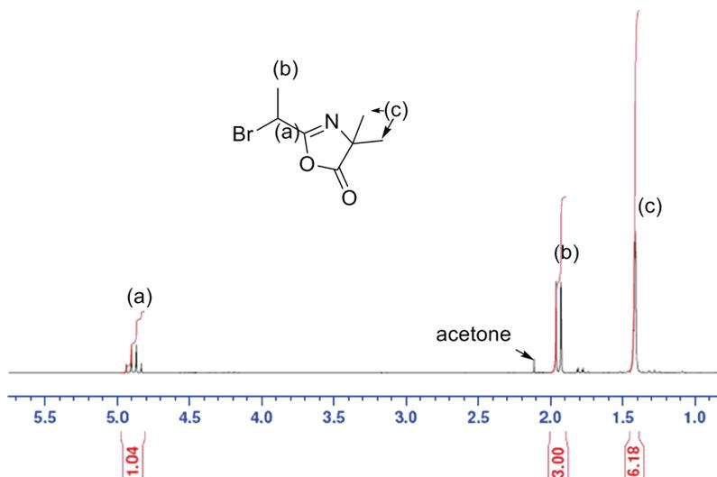
Figure 17:  $^1\text{H}$  NMR spectrum of 2-(1-bromoethyl)-4,4-dimethyl-4H-oxazolin-5-one (2) in  $\text{CDCl}_3$ .
