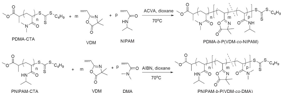
*Scheme 2: Synthesis of PDMA-*b*-P(VDM-co-NIPAM) and of PNIPAM-*b*-P(VDM-co-DMA) copolymers by RAFT polymerization.*
