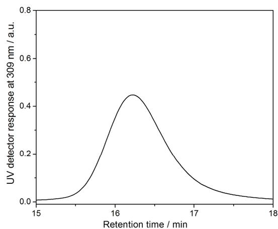
Figure 11: SEC trace of the 4-fluorobenzylamine-terminated PNIPAM ( $M_{n,SEC} = 6460$  g.mol<sup>-1</sup>; PDI = 1.04) using UV detection at 309 nm.
