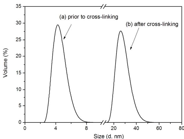
*Figure 10: Particle sizes from dynamic light scattering of PDMA<sub>23</sub>-*b*-P(VDM<sub>10</sub>-*co*-NIPAM<sub>46</sub>) copolymers in water at 25°C: (a) prior to cross-linking and, (b) after cross-linking of self-assembled structures with 2,2'-ethylenedioxybis(ethylamine).*
