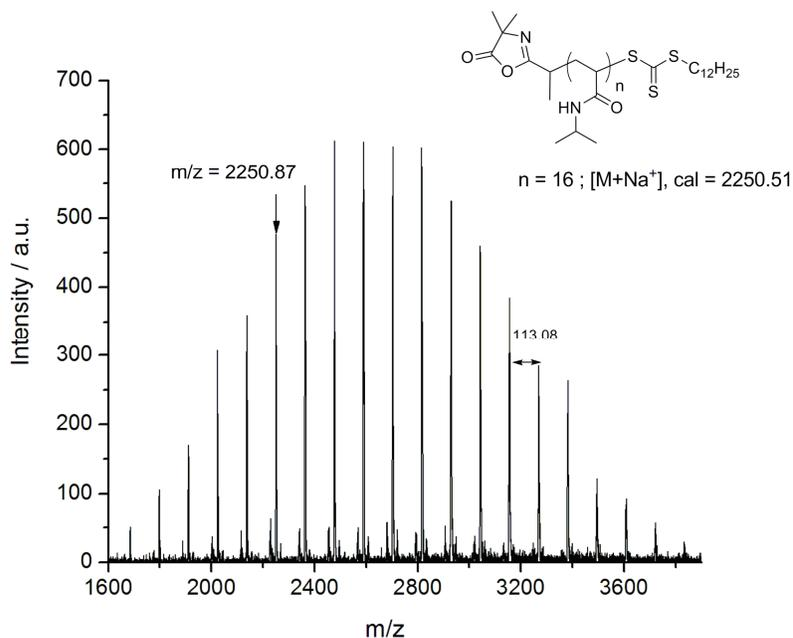
Figure 9: MALDI-TOF mass spectrum of a PNIPAM synthesized by RAFT polymerization using the azlactone-functionalized trithiocarbonate (**3**) as the RAFT agent and ACVA as the initiator in dioxane at  $70^\circ\text{C}$  ( $[\text{NIPAM}]_0/[\text{3}]/[\text{ACVA}]_0 = 17/1/0.1$ ; 72% monomer conversion;  $M_{n,SEC} = 3400 \text{ g}\cdot\text{mol}^{-1}$ ;  $\text{PDI} = 1.07$ ). Matrix: *trans*-2-[3-(4-*tert*-butylphenyl)-2-methyl-2-propenylidene]malononitrile (DCTB), sodium trifluoroacetate.
