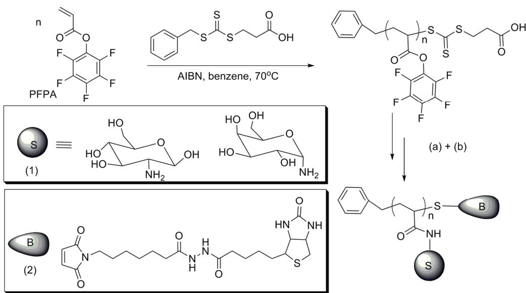
*Scheme 63: Synthesis of PPFPA by RAFT polymerization and the subsequent one-pot synthesis of glycopolymers . Conditions: (a) nucleophilic substitution of sugar amine (1) in DMF–water (50/50 vol%) at room temperature, (b) in-situ aminolysis of the RAFT end-group and the thiol-ene reaction using biotin modified maleimide (2).*
