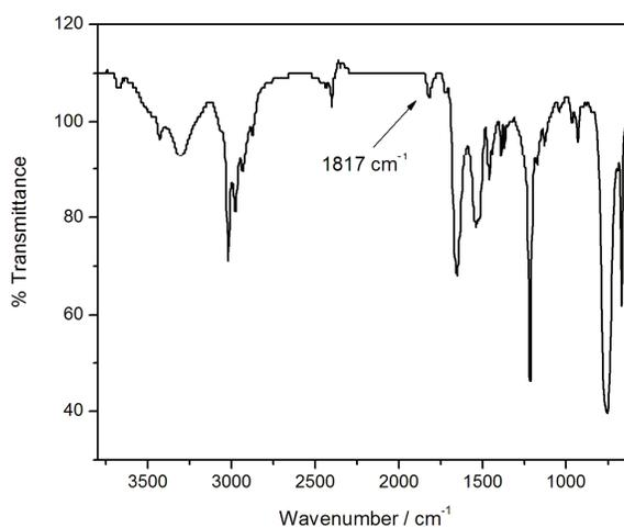
Figure 11: FT-IR spectrum of azlactone-terminated PEO<sub>44</sub>-*b*-PNIPAM<sub>101</sub> diblock copolymer.
