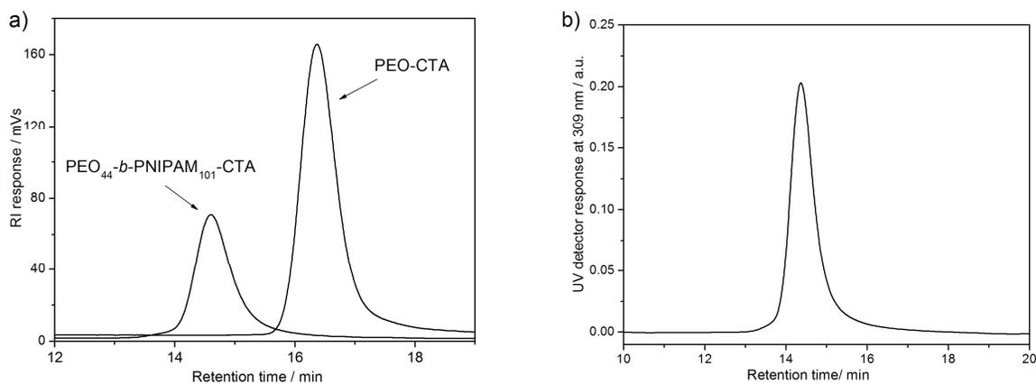
Figure 6: a) Overlay of SEC traces of PEO<sub>44</sub>-*b*-PNIPAM<sub>101</sub> and PEO-CTA using RI detection and, b) extracted UV chromatogram at 309 nm of PEO<sub>44</sub>-*b*-PNIPAM<sub>101</sub>.
