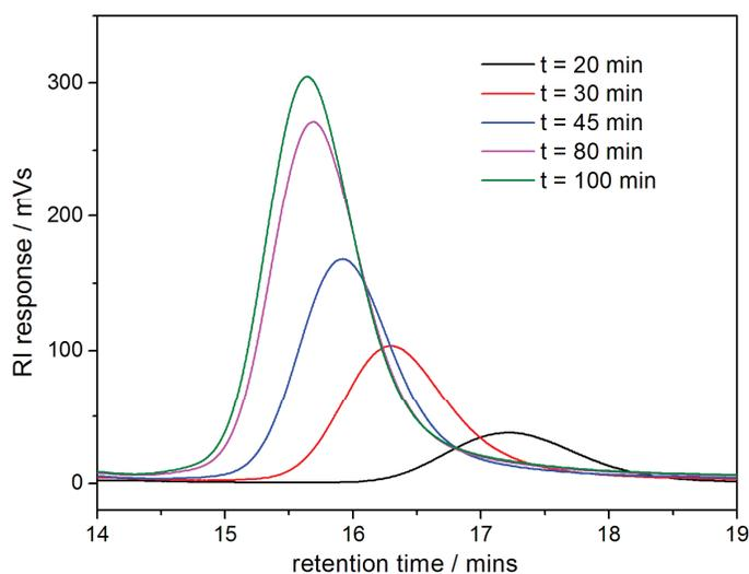
Figure 7: Evolution of the normalized SEC traces of PNIPAMs with time for the RAFT polymerization of NIPAM using ACVA as the initiator and the azlactone-functionalized trithiocarbonate (**3**) as the RAFT agent in dioxane at 70°C,  $[NIPAM]_0:[\mathbf{3}]_0:[ACVA]_0 = 55:1:0.1$ .
