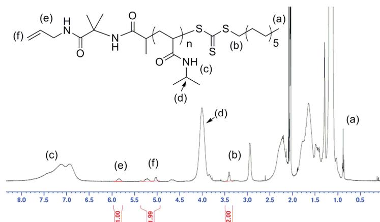
Figure 13:  $^1\text{H}$  NMR spectrum (solvent: acetone  $D_6$ ) of the polymer obtained after reacting the  $\alpha$ -azlactone- $\omega$ -dodecyltrithiocarbonate PNIPAM with allyl amine at room temperature in THF for 24h.
