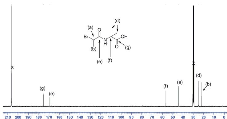
Figure 16:  $^{13}\text{C}$  NMR spectrum of 2-(2-bromopropionylamino)-2-methyl-propanoic acid (**1**) in acetone  $D_6$ .
