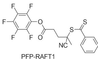
*Scheme 69: Structure of PFP-functionalized RAFT agent: PFP-RAFT1.*
