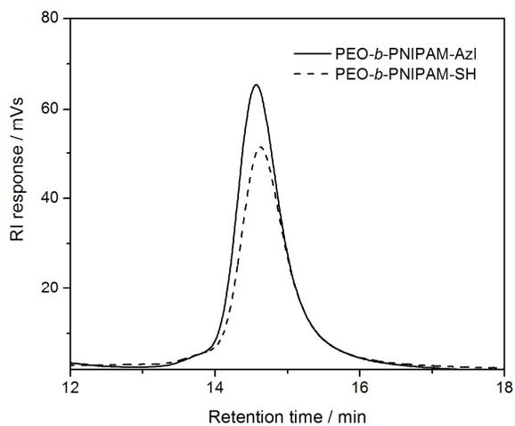
Figure 10: Overlay of SEC traces of PEO<sub>44</sub>-*b*-PNIPAM<sub>101</sub>-SH before (---) and after (—) coupling with VDM in the presence of DMPP in THF at 25°C.
