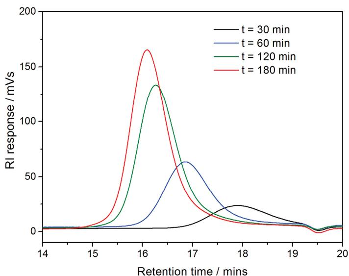
*Figure 6: Evolution of the normalized SEC traces of PEAs with time for the RAFT polymerization of EA using ACVA as the initiator and the azlactone-functionalized trithiocarbonate (**3**) as the RAFT agent in dioxane at 70°C,  $[\text{EA}]_0/[(\mathbf{3})]_0/[\text{ACVA}]_0 = 50:1:0.1$ .*
