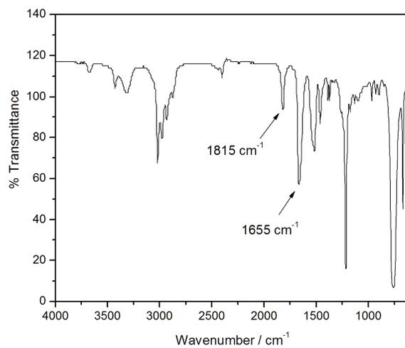
Figure 5: FT-IR spectrum of  $\text{PEO}_{44}\text{-}b\text{-}P(\text{VDM}_{18}\text{-}co\text{-}NIPAM_{130})$  block copolymer.
