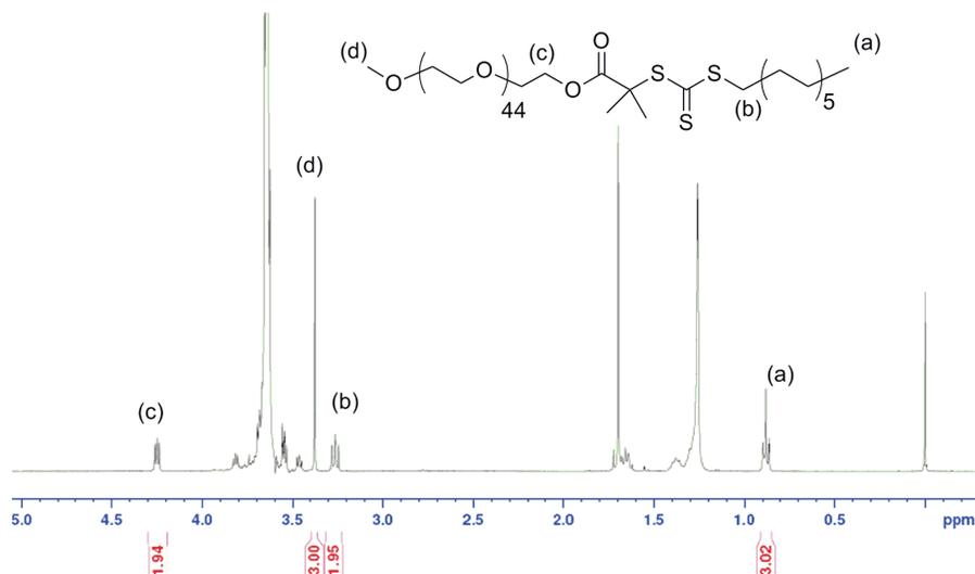
Figure 2: <sup>1</sup>H NMR spectrum of PEO-CTA in CDCl<sub>3</sub>.
