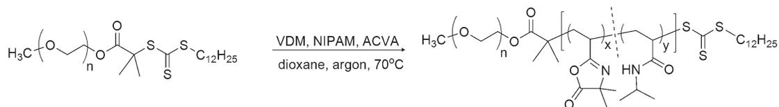
Scheme 3: RAFT copolymerization of VDM and NIPAM using PEO-CTA as the macromolecular chain transfer agent and using ACVA as the initiator in dioxane at  $70^\circ\text{C}$ .
