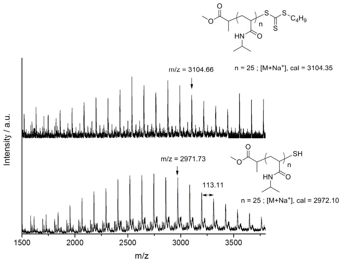
Figure 6: MALDI-TOF mass spectra for PNIPAM-CTA (top) and PNIPAM-SH (bottom).
