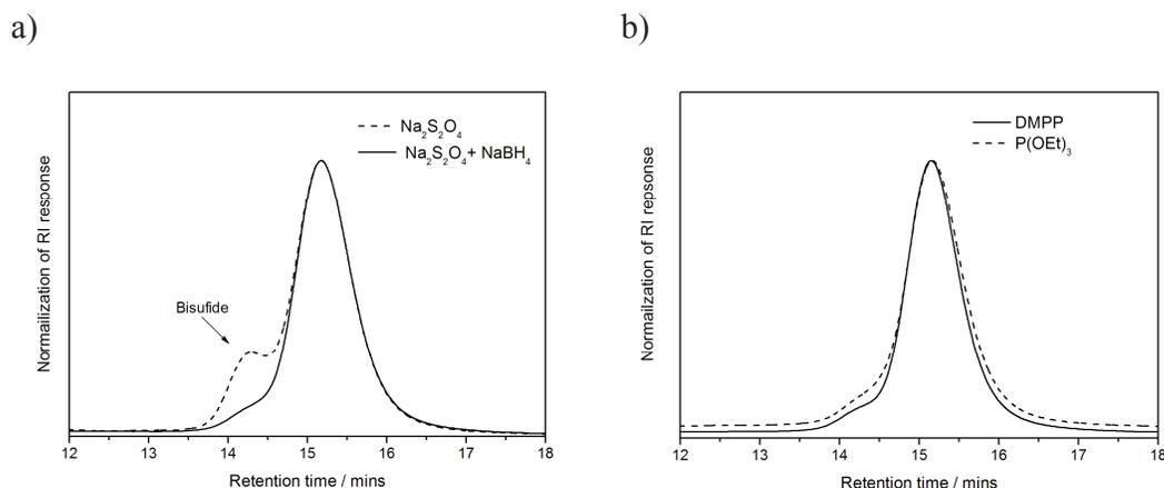
Figure 4: SEC traces of polymers resulting from the aminolysis of PNIPAM-CTA ( $M_{n,SEC} = 15070 \text{ g}\cdot\text{mol}^{-1}$ ;  $PDI = 1.06$ ) in tetrahydrofuran (THF) at room temperature: a) using  $\text{Na}_2\text{S}_2\text{O}_4$  and the mixture  $\text{Na}_2\text{S}_2\text{O}_4/\text{NaBH}_4$  as reducing agents, b) using  $\text{P}(\text{OEt})_3$  and DMPP as reducing agents.
