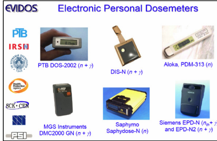
Figure 1.7: Electronic neutron personal dosimeters investigated in the EVIDOS survey.
