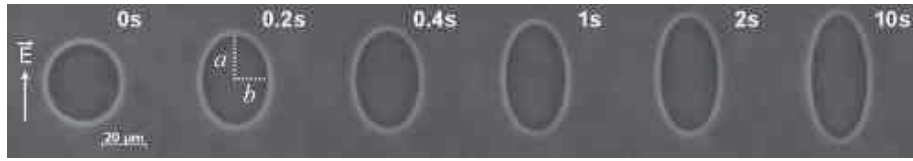
Figure 1.31: Irradiation of a GUV containing X_{porph} = 0.03 in the presence of an AC field (10 V, 1 MHz), which induces prolate deformation. The electric field direction is indicated on the left and the irradiation time on top of each snapshot. The scale bar represents 20 \mu\text{m} [57].
