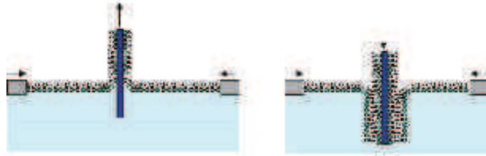
Figure 2.9: Scheme of the Langmuir-Blodgett deposition technique. The glass slide is taken out of the water subphase, inducing the deposition of a first lipid monolayer. By returning to the water phase and crossing a second time the interface, a second monolayer is deposited, leading to a supported bilayer.
