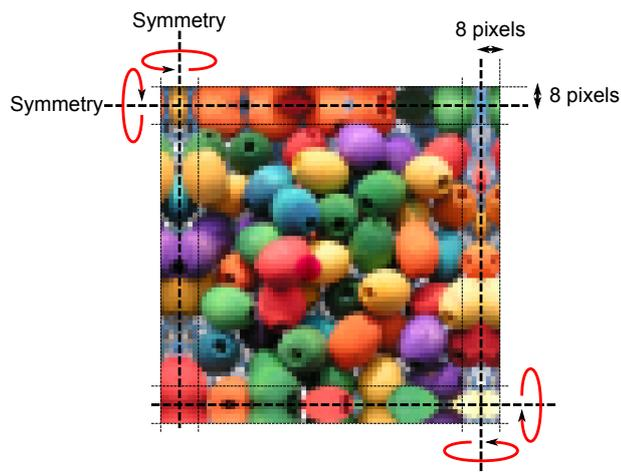
Figure 5.9: Image extension by symmetry for border handling
