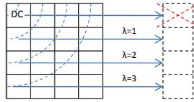
Figure 6.22: Descriptor computed on a 4x4 DCT block.
