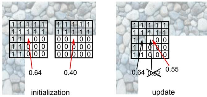
Figure 6.27: Confidence map order. Confidences  $w_a$ ,  $w_b$  and  $w_c$  are computed for center pixels using neighboring confidences. At initialization,  $w_a = 0.64$  for instance. After synthesizing pixel a,  $w_b$  is updated by assigning  $w_a^1$ .
