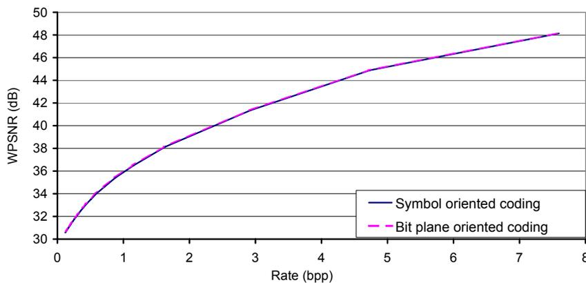
Figure 3.12: Compression ratios of QM encoding for both symbol oriented and bit plane oriented QM Coding
