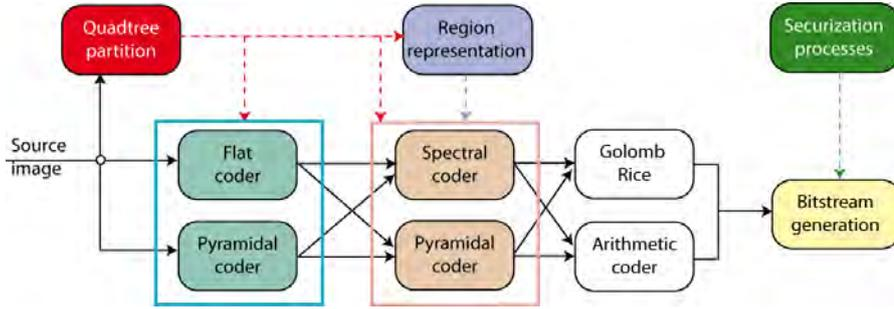
Figure 2.5: Block diagram of extended LAR coder profile
