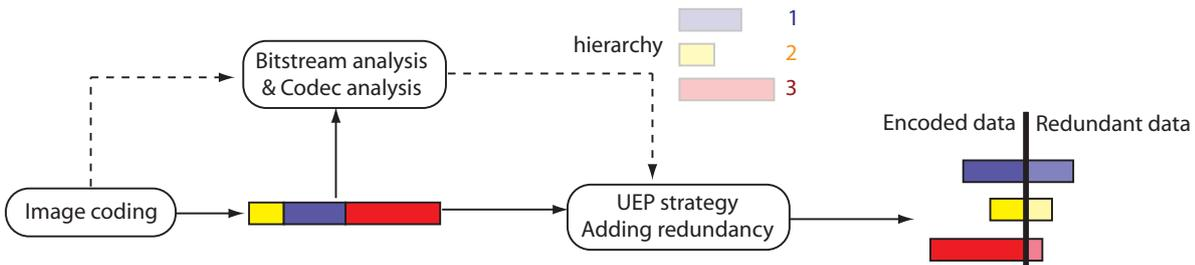
Figure 4.8: UEP principles: hierarchy and redundancy
