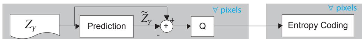
Figure 3.7: QM coding scheme with bit plane orientation
