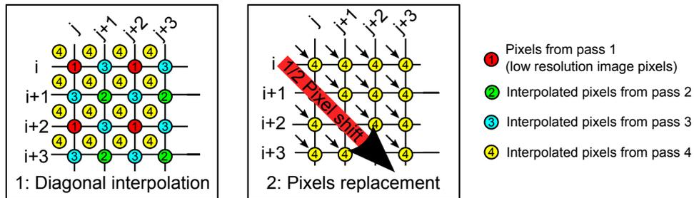
Figure 5.7: Step 4: diagonal interpolation for 1/2 pixel shifting
