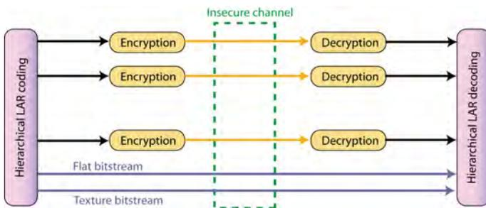
Figure 4.3: Interleaved S+P hierarchical selective encryption principle
