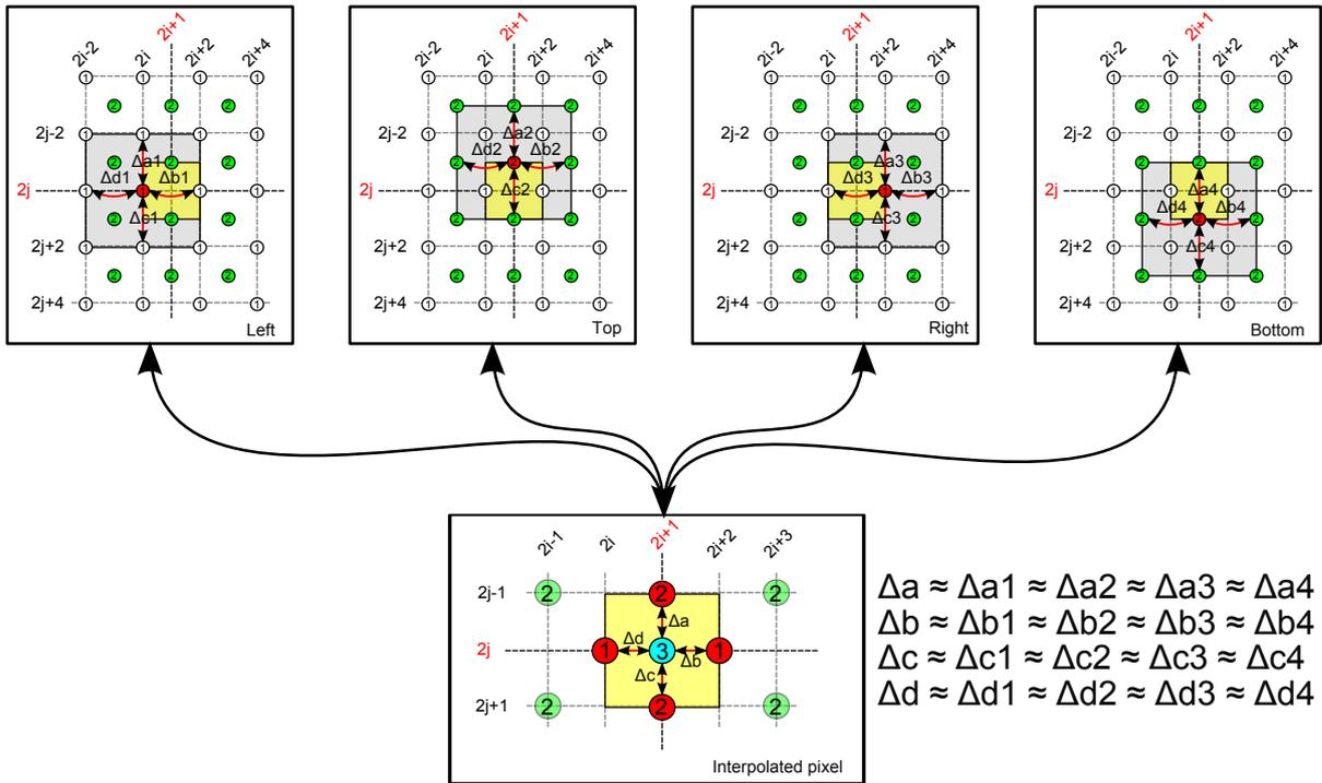
Figure 5.6: Step 3 - vertical / horizontal interpolation
