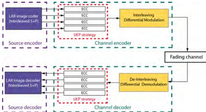
Figure 4.9: Overall layout of the multi-layer transmission/compression system
