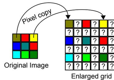
Figure 5.4: Step 1 - Pixel copy over an enlarged grid
