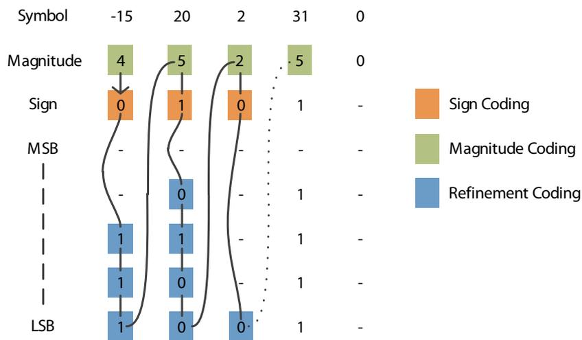
Figure 3.10: Example of QM coding with symbol orientation
