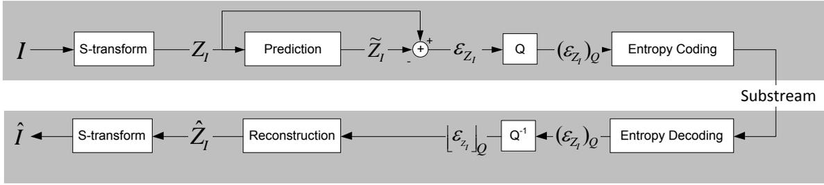
Figure 3.1: Interleaved S+P Coding of a resolution level
