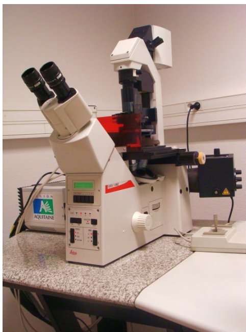
Figure 2.10: Leica DMIRE confocal laser scanning microscope used at CRPP for FRAP experiments in this work.
