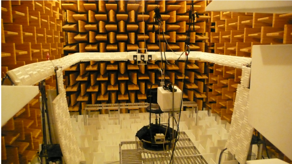
Figure 5: Example of the experimental setup for recording HRTFs in an anechoic chamber. The listener is seated at the centre of the chamber with microphones in both ear canals while the mechanical arm with speakers attached moves up and down for different elevations. Different locations in azimuth are recorded by rotating the chair the listener is seated on.
