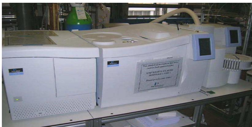
**Figure B-II-3 : Appareil de GC-MS Clarus 500 (PerkinElmer).**
