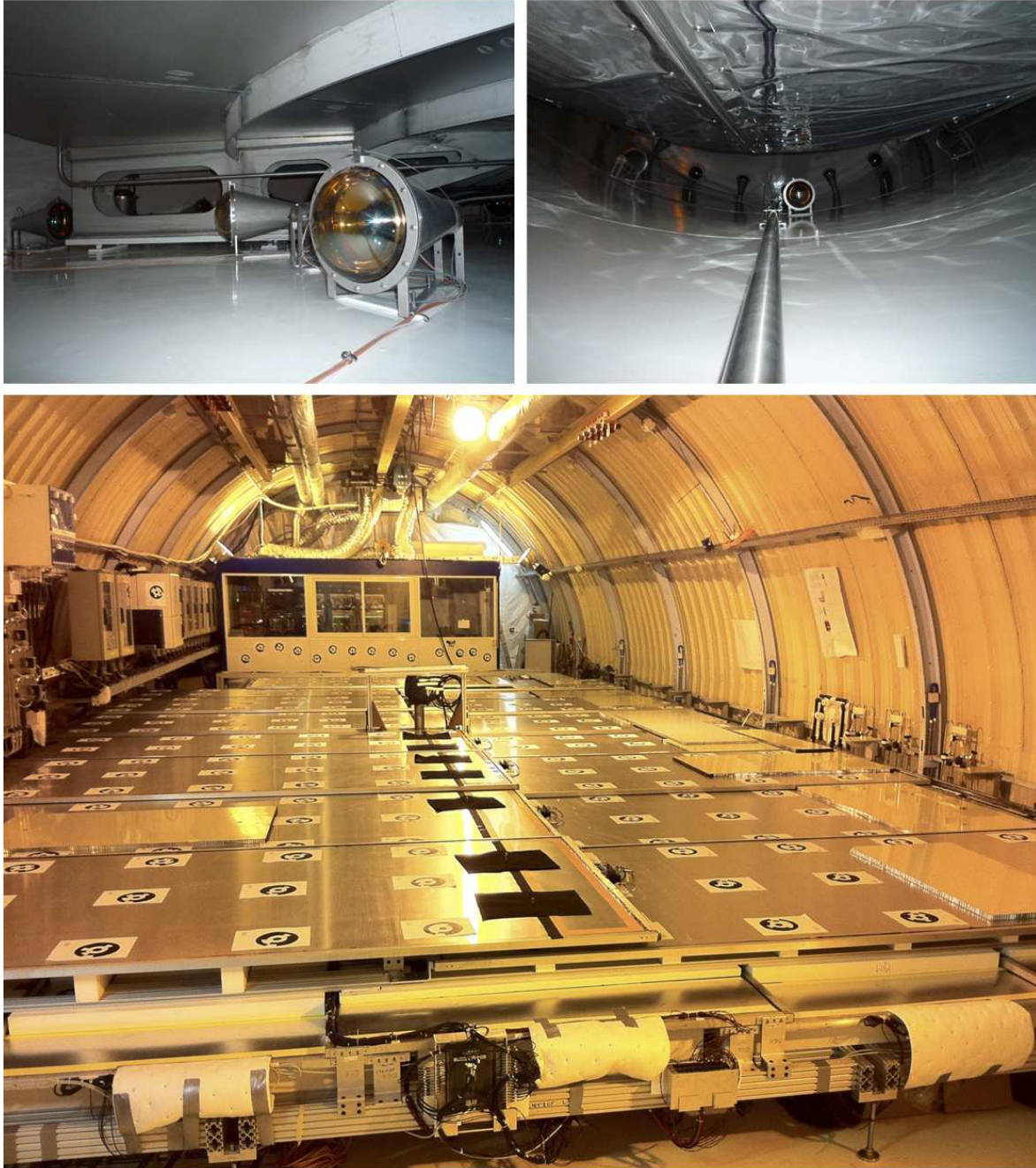
Figure 3.13: (top) Inside of the inner veto volume. IV PMTs with their peculiar orientation and the reflective foils and white paint on the IV wall are visible. (bottom) Outer veto fully mounted above the detector, at the ground level.
