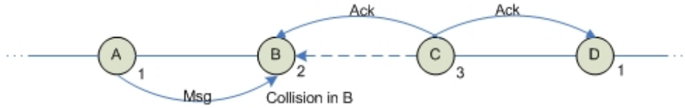
Figure 4.25: Type 4 color conflict between A and D causing a collision in B .
