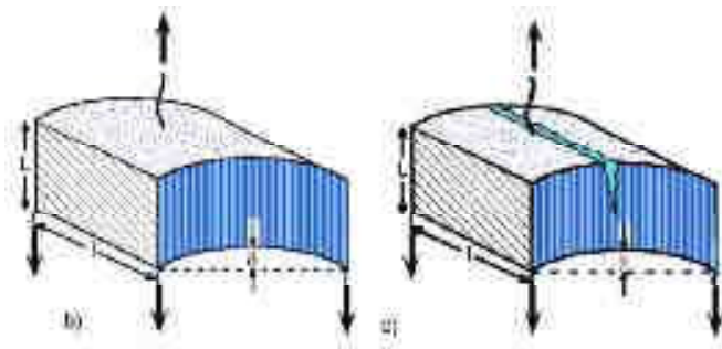
Figure IV-11: Deformation mechanisms of UHMWPE after yield point with lamellae bending [1]
