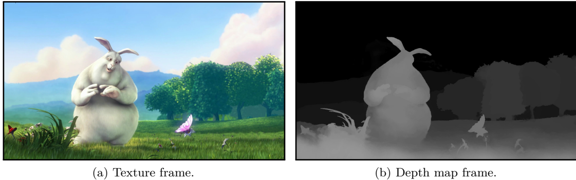
Figure 2.3: One frame of a 2D plus depth video sequence. Darker is farther.
