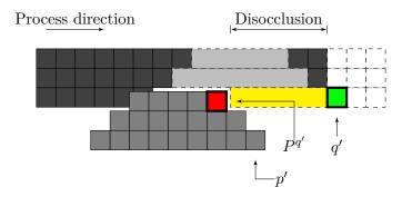
(c) Details of some rows of pixels in the synthesized view for a non rectified projection.
