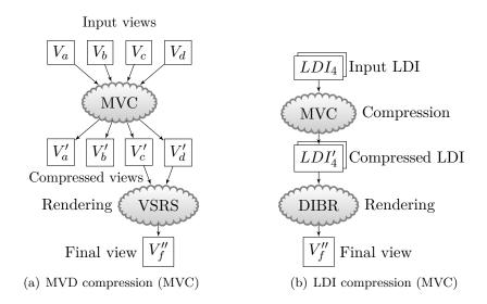
Figure 6.19: Block-diagrams of the two compared compression schemes. Figure 6.19(a) presents the classical multi-view compression scheme, using the MVC codec from MPEG [Tanimoto et al., 2008]. Figure 6.19(b) shows the proposed LDI compression scheme also using the MVC codec.
