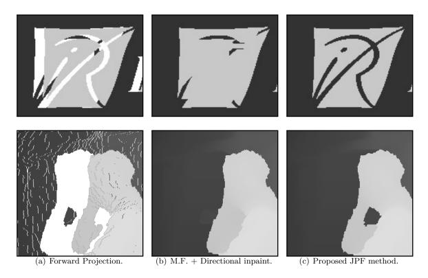
Figure 4.4: Virtual depth map synthesized by three forward projection methods. The point-based projection method generates cracks and disocclusions 4.4(a). Median filtering and directional inpainting [Nguyen et al., 2009] fills some holes with foreground depth 4.4(b). The proposed JPF method fills cracks and disocclusions with realistic background 4.4(c).
