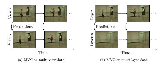
Figure 6.1: Block-diagrams of the configuration of MVC codec for compressing 3D sequences. In Fig 6.1(a), MVC is used with multi-view sequence to exploit both temporal and inter-view correlations. In Fig 6.1(b), MVC is used with sequence of LDI to exploit both temporal and inter-layer correlations.
