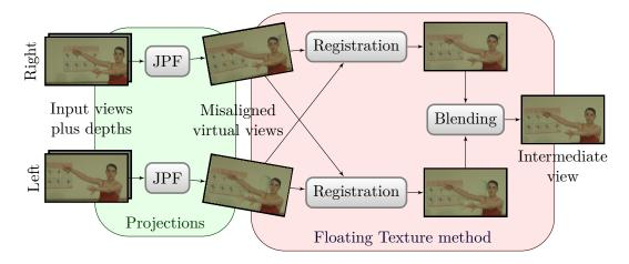
Figure 4.11: Floating Texture scheme for intermediate view synthesis. Each input view is projected onto the virtual viewpoint, using the Joint Projection Filling (JPF) method to fill in disocclusions and preserve contours. Projected views are realigned with the Floating Texture algorithm, then blended together with a weighting based on the virtual view position and confidence score.
