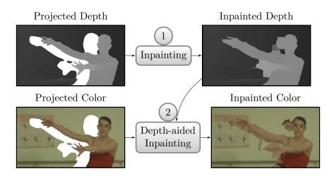
Figure 3.9: Depth-aided inpainting scheme [Daribo & Pesquet, 2010]. Firstly, the depth map is inpainted with a Navier-Stokes based algorithm [Bertalmío et al., 2001]. Secondly, the texture is inpainted, aided with the resulting depth map.
