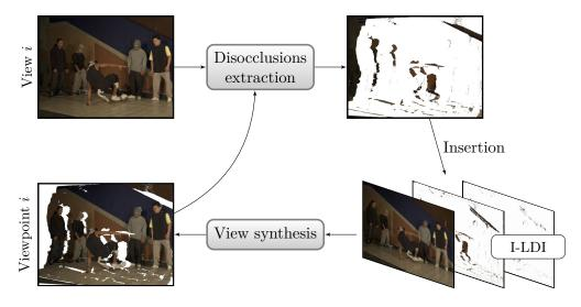
Figure 6.5: Step of I-LDI construction for view i, with residual information extraction.
