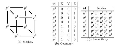
Figure 2.8: VRML representation of a simple cube mesh.
