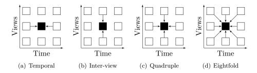
Figure 2.11: Various prediction schemes for MVC frames [Merkle et al., 2007]. Both temporal predictions 2.11(a) and inter-view predictions 2.11(b) can be associated in quadruple 2.11(c) or eightfold 2.11(d) prediction scheme.
