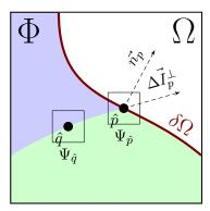
Figure 3.6: Notation diagram, introduced in [Criminisi et al., 2003]. Given the block  $\Psi_p$ ,  $n_p$  is the normal to the contour  $\delta\Omega$  separating the hole region  $\Omega$  from the non-hole region  $\Phi$ .  $\Delta I_p^{\perp}$  is the isophote at point p.
