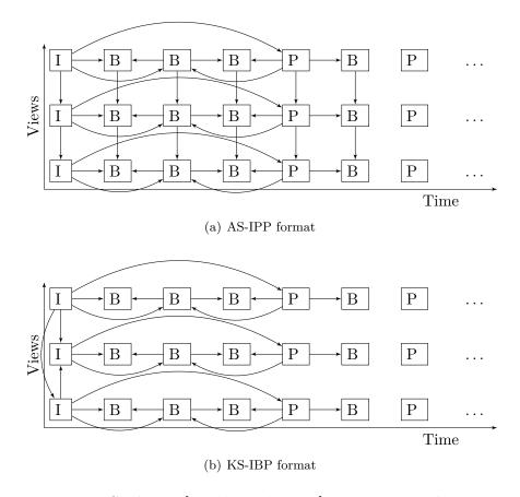
Figure 2.13: Various MVC schemes [Merkle et al., 2007]. Inter-view prediction may be used to predict all frames 2.13(a), or only key frames 2.13(b).
