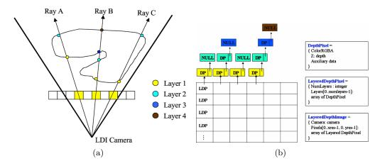
Figure 5.1: Structure of a Layer Depth Image (LDI) (from [Yoon et al., 2007]).
