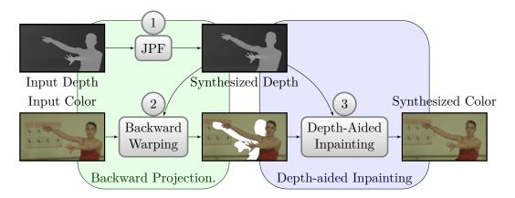
Figure 4.5: Proposed scheme for virtual view extrapolation from single input view plus depth sequence. First, the Joint Projection Filling (JPF) method handles cracks and disocclusions during the depth map warping. Then, the backward projection method synthesizes the virtual view. Finally, the depth-aided inpainting takes into account the high quality of the computed depth map to fill disoccluded areas in the synthesized view.
