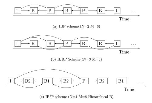
Figure 2.9: Classical GOP structures. Each arrow represents a prediction. Anchor frames can be separated by one 2.9(a), two 2.9(b), or more B-frames. B-Frames can be organized in a hierarchical structure 2.9(c).
