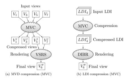
Figure 6.2: Block-diagrams of the two compared compression schemes. Figure 6.2(a) presents the classical multi-view compression scheme, using the MVC codec from MPEG [Tanimoto et al., 2008]. Figure 6.2(b) shows the proposed LDI compression scheme, using the MVC codec on different layers.
