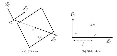
Figure 3.1: Pinhole camera coordinate system  $\mathcal{R}_C$  with its image plane coordinates system  $\mathcal{I}_C$ .
