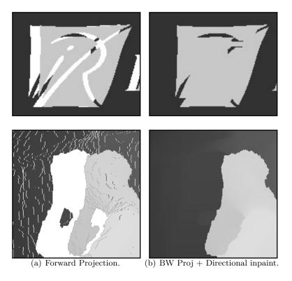
Figure 3.8: Results of virtual depth map synthesis. The point-based projection method generates cracks and disocclusions 3.8(a). Median filtering and directional inpainting [Nguyen et al., 2009] fill some holes with foreground depth 3.8(b).
