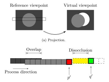
(b) Details of a single row of pixels in the synthesized view for a rectified projection.
