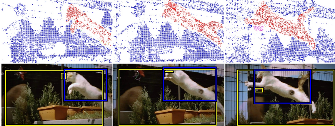
Figure 4.4: Localizing objects in videos. (Top) Results of the motion segmentation. (Bottom) Tubes fit to the motion segments (the one selected by our approach is in blue).
