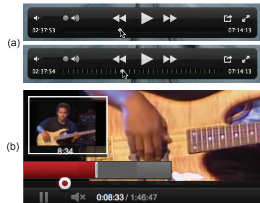
Figure 2: Manipulating visual space to increase pointing accuracy: (a) dwelling while dragging the OS X QuickTime Player 10.1 timeline slider zooms the timeline in to provide 1 second precision in a 10 second window; (b) some YouTube videos have a Focus+Context timeline with a secondary slider providing 1 second precision.
