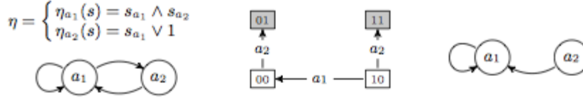
Fig. 2. An interaction network, its state graph and the corresponding regulation graph.
