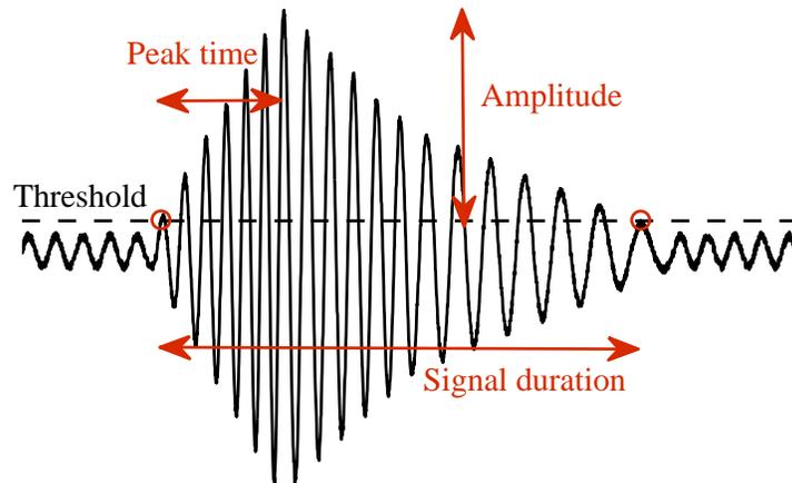
Figure 3.11: Scheme of an AE waveform
