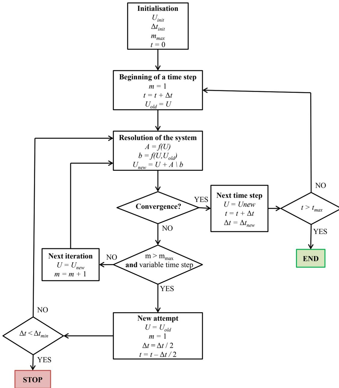
Figure B.1: Algorithm of the finite-element simulation code
