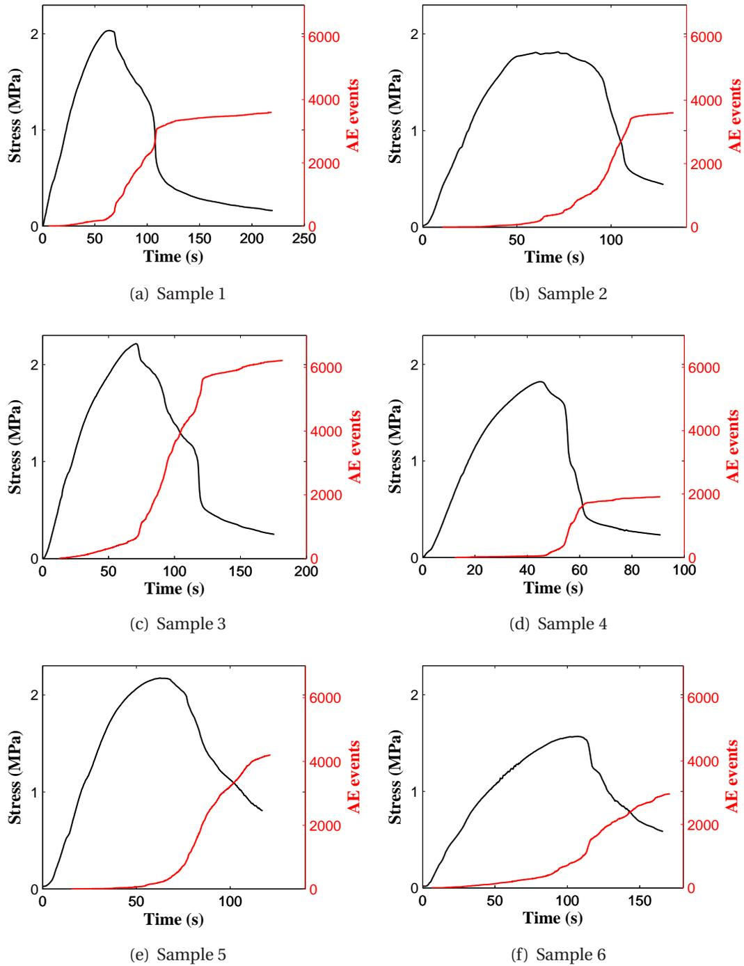
Figure 3.8: Stress-strain profiles and cumulative AE signal distributions
