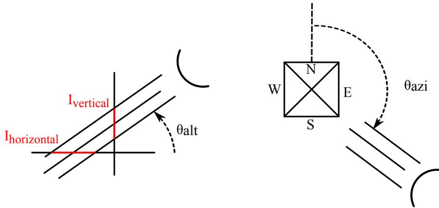
Figure 5.7: Calculation procedure of the direct solar radiation
