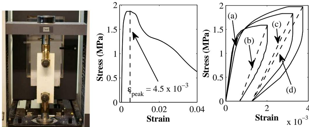
Figure 2.4: Stress-strain profiles on a full tensile loading (left) and on three tests interrupted before peak strain (right): (a)  $E_0 = 2750$  MPa, (b)  $E_e = 1170$  MPa, (c)  $E_e = 859$  MPa, (d)  $E_e = 782$  MPa
