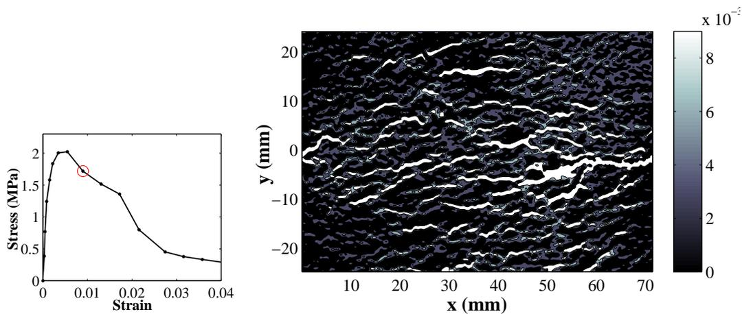
Figure 3.5: Example of a longitudinal strain mapping
