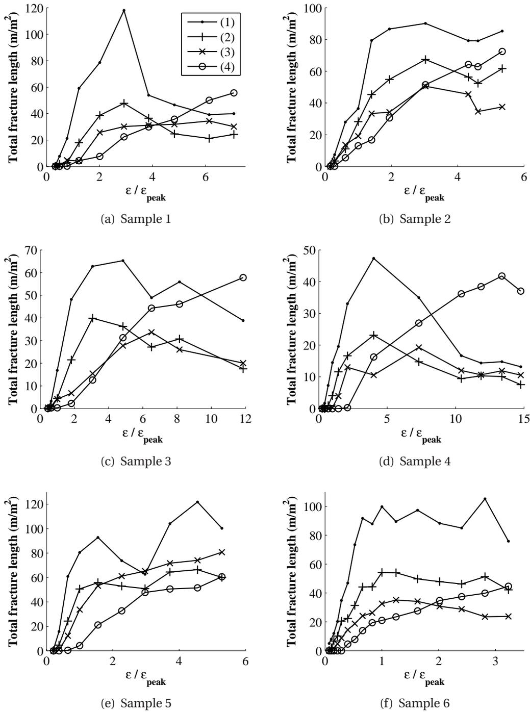
Figure 3.7: Visible fracture length per square meter of sample surface : (1)  $3 \leq w < 5 \mu\text{m}$ , (2)  $5 \leq w < 10 \mu\text{m}$ , (3)  $10 \leq w < 50 \mu\text{m}$ , (4)  $w \geq 50 \mu\text{m}$
