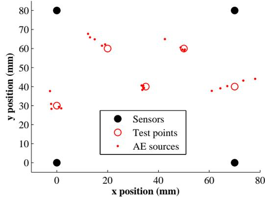
Figure 3.3: Accuracy testing of the localisation procedure
