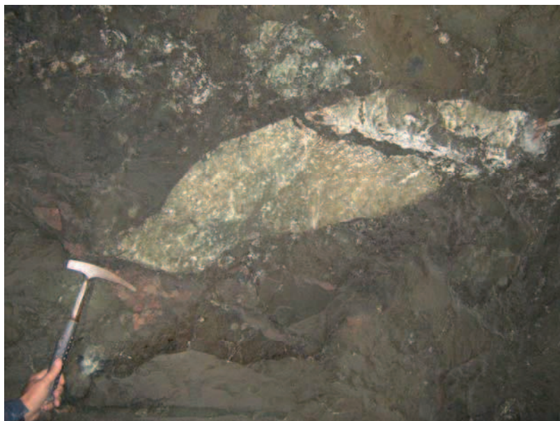
Fig. B-3: Marble fragments within strongly altered basalt, suggesting mafic magma stoning. The photo was taken in the gallery, about 200m underground. Reddish ribbons consist in K-feldspar occurrence due to the development of potassium metasomatism.
