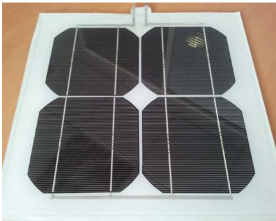
Figure 5.11. PV modules issued from HJ solar cells to be tested at the laboratory and for outdoor operation.
