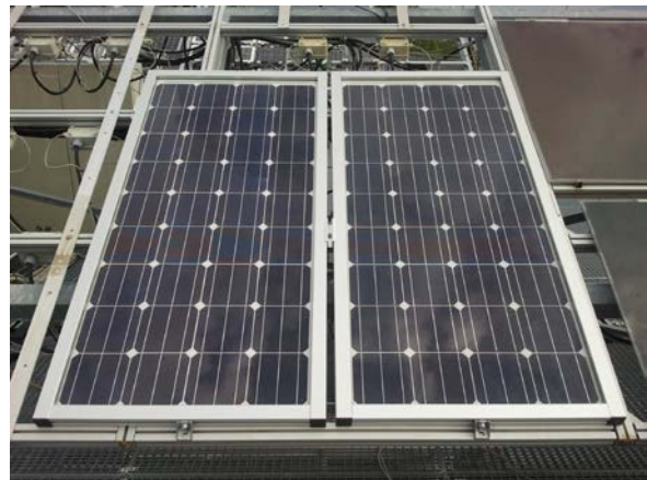
Figure 5.11. PV modules issued from HJ solar cells to be tested at the laboratory and for outdoor operation.
