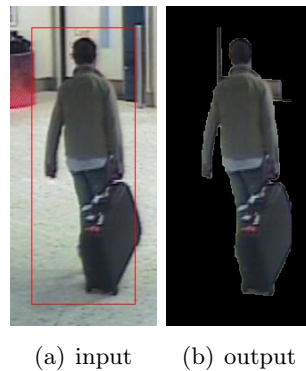
Figure 4.3: GrabCut: the red rectangle can be given either by a user or by a human detector.
