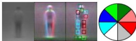
Figure 3.5: Mean human image with corresponding edge magnitudes and the 15 most dominant cells. From the left: the first image shows the mean human image calculated over all positive samples in the database; the second image shows the corresponding mean edge magnitude response; the third image shows this later image superposed with the 15 most dominant cells of size 8 \times 8 pixels. The cell bounding boxes are drawn with a color set by their most dominant edge orientation with the scheme defined in the last image.
