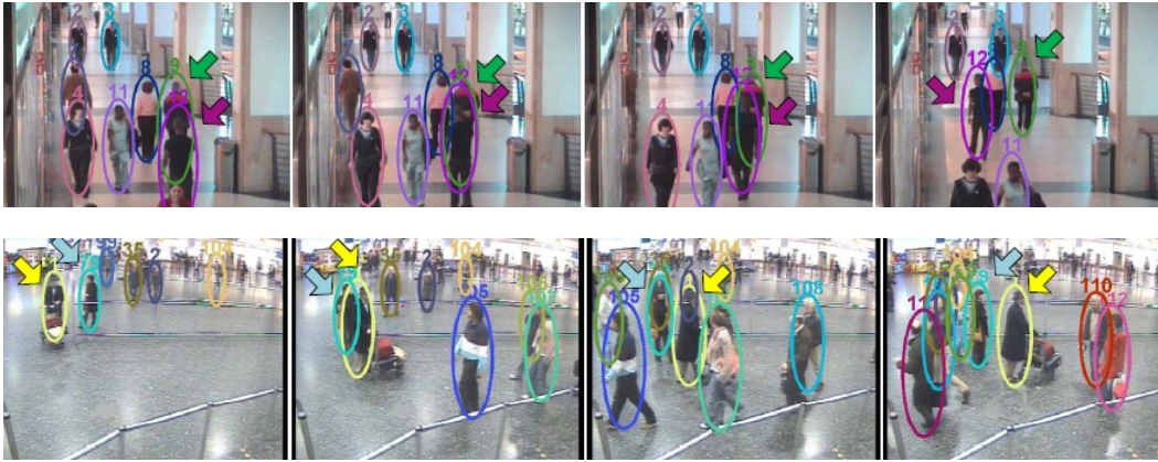
Figure 3.9: Example of tracking results on CAVIAR (top row) and i-LIDS (bottom row) dataset [Kuo 2010].
