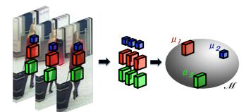
Figure 5.14: Computation of three MRC patches. Covariances gathered from tracking results are used to compute the mean covariance using Riemannian manifold space (depicted with the surface of the sphere). The mean covariance forms MRC patch.
