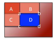
Figure 5.3: Calculation of the pixel sum of rectangle D. This can be done with four array references: a, b, c, d are the values of the integral image at given positions. Thus, a = s(A), b = s(A) + s(B), c = s(A) + s(C), d = s(A) + s(B) + s(C) + s(D). The sum within D can be computed as s(D) = d + a - b - c.
