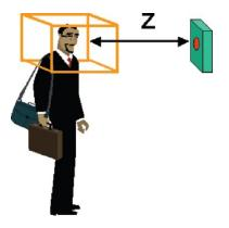
Figure 2.2: Illustration of standoff (Z), capture volume, and residence time. The recognition device is at the far right of the illustration. The capture volume is represented as a box around the subject's head [Matey 2008].
