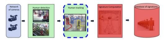
(a) the processing chain of an automatic human signature generation
