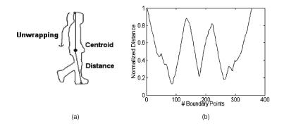
Figure 2.5: Silhouette representation [Wang 2003]: (a) illustration of boundary extraction and counter-clockwise unwrapping and (b) the normalized distance signal consisting of all distances between the centroid and the pixels on the boundary.
