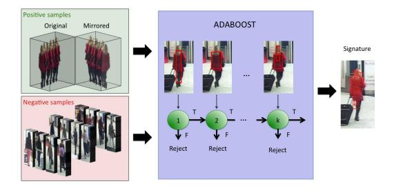
Figure 5.4: Haar signature: cascade of k strong classifiers. At each stage a new strong classifier is trained to eliminate additional negatives, requiring additional computation.
