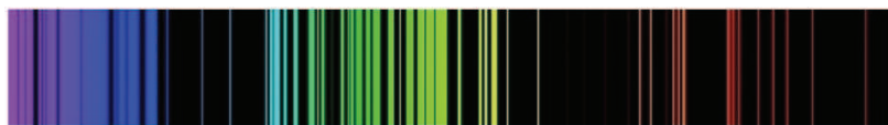
Figure 2.3.4: Emission spectrum of iron in the visible range. In total 4757 emission lines related to iron atomic emission were recorded between 200 and 1000 nm [NIST Atomic Spectra Database Lines].
