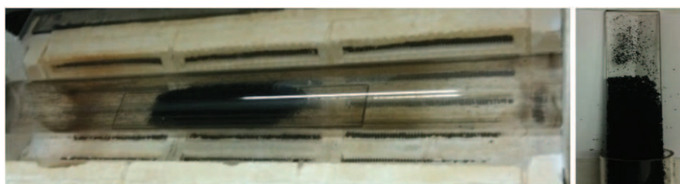
Figure 5.1.6: Pictures showing the very clean quartz tube and the quartz plate supporting the ceramic \mu -particles right after 10 min CNT growth by aerosol-assisted CVD at low temperature [31].
