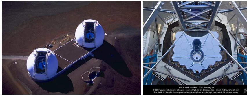
Figure 1.12 : The Keck twin telescopes and one of their segmented primary mirror (credit Keck Observatory).
