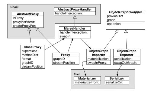
Figure 8.1: Simplified UML class diagram of Marea.
