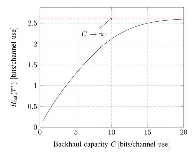
Figure 3.7: Net ergodic achievable rate  $R_{\rm net}(\overline{\tau}^*)$  with optimal channel training  $\overline{\tau}^*$  vs backhaul capacity C for SNR = 10 dB and T = 1000.
