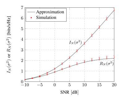
Figure 3.24: Comparison of the average normalized mutual information  $I_N(\sigma^2)$  and the normalized rate with MMSE decoding  $R_N(\sigma^2)$  with their deterministic approximations  $\bar{I}_N(\sigma^2)$  and  $\bar{R}_N(\sigma^2)$ . Error bars represent one standard deviation in each direction.
