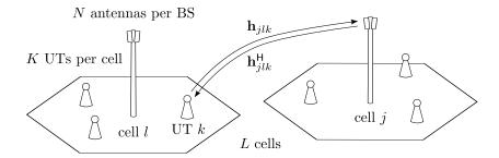
Figure 3.10: System model: In each of the L cells is one BS and K UTs. The BSs are equipped with N antennas. We assume channel reciprocity, i.e., the downlink channel  $\mathbf{h}_{jlk}^{\mathsf{H}}$  is the complex conjugate transpose of the uplink channel  $\mathbf{h}_{jlk} \in \mathbb{C}^N$ .
