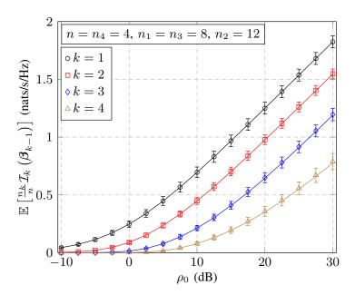
Figure 3.19: Average normalized mutual information  $\mathbb{E}\left[\frac{n_k}{n}\mathcal{I}_k(\boldsymbol{\beta}_{k-1})\right]$  after the kth hop versus the transmit SNR  $\rho_0$  of the source node. The deterministic equivalents  $\frac{n_k}{n}\bar{\mathcal{I}}_k\left(\bar{\boldsymbol{\beta}}_{k-1}\right)$  are drawn by solid lines, the simulation results by markers. The error bars correspond to one standard deviation of the simulation results in each direction.
