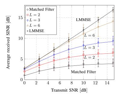
Figure 3.8: Average received SINR versus SNR at the output of the matched filter, LMMSE detector and the polynomial expansion detector with approximate weights for different values of L. Markers correspond to simulation results, solid lines to the deterministic SINR approximations. Error bars indicate one standard deviation of the simulation results in each direction.
