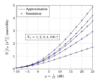
Figure 3.16: Ergodic mutual information  $\mathbb{E}\left[I_N(\sigma^2)\right]$  of the multi-keyhole channel and its deterministic equivalent  $\bar{I}_N(\sigma^2)$  versus  $\rho=\frac{1}{\sigma^2}$ .
