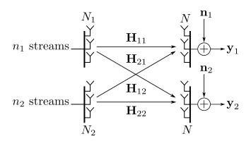
Figure 3.25: Interference channel from two transmitters with  $N_k$  (k=1,2) antennas, respectively, to two receivers with N antennas each. Each transmitter sends  $n_k$  independent data streams to its respective receiver.
