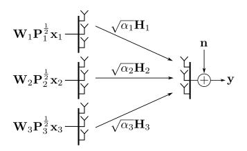
Figure 3.23: MIMO MAC from three transmitters (k = 1, 2, 3) with  $N_k$  antennas to a receiver with N antennas. Each transmitter sends  $n_k$  streams with precoding matrix  $\mathbf{W}_k$  and power allocation  $\mathbf{P}_k$  over the channel  $\sqrt{\alpha_k}\mathbf{H}_k$ .
