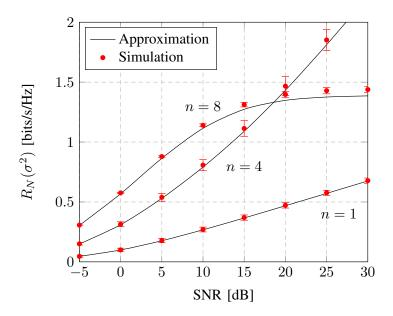
Figure 3.22: Sum rate  $R_N(\sigma^2)$  at the output of the MMSE decoder for user 2 versus SNR for different numbers of transmit signatures n, N = 16,  $N_i = 8$ ,  $\mathbf{P}_i = \mathbf{I}_n$ ,  $\alpha = 0.5$ . Error bars represent one standard deviation on each side.
