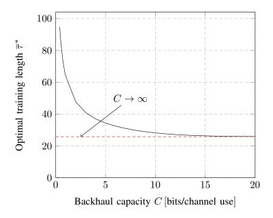
Figure 3.6: Optimal training length  $\overline{\tau}^*$  vs backhaul capacity C for SNR = 10 dB and T=1000.
