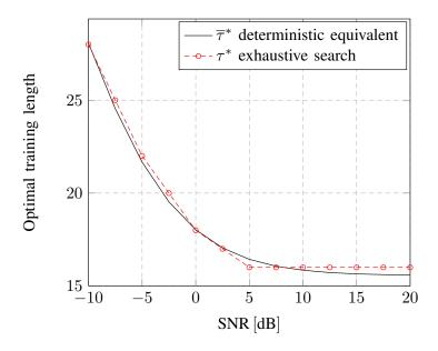
Figure 3.5: Optimal training length  $\tau^*$  and  $\overline{\tau}^*$  vs SNR for C=1 bits/channel use and T=100. The solid line corresponds to  $\overline{\tau}^*$  maximizing  $\overline{R}_{\rm net}(\tau)$ , the dashed line corresponds to  $\tau^*$  maximizing  $R_{\rm net}(\tau)$  and is obtained by an exhaustive search based on Monte Carlo simulations.
