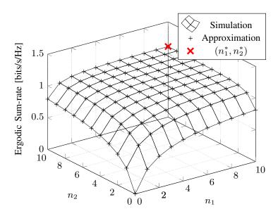
Figure 3.26: Sum-rate versus number of transmitted data-streams  $(n_1, n_2)$  for SNR = 0 dB and all other parameters as provided in Table 3.2. Solid lines correspond to simulation results, markers to the deterministic approximation by Theorem 23 (ii). As expected, both transmitters should send the maximum number of independent streams.
