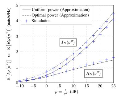
Figure 3.17: Ergodic mutual information  $\mathbb{E}\left[I_N(\sigma^2)\right]$  and sum-rate  $\mathbb{E}\left[R_N(\sigma^2)\right]$  of the multiple access channel and their asymptotic approximations  $\bar{I}_N(\sigma^2)$  and  $\bar{R}_N(\sigma^2)$  versus  $\rho=\frac{1}{\sigma^2}$ .
