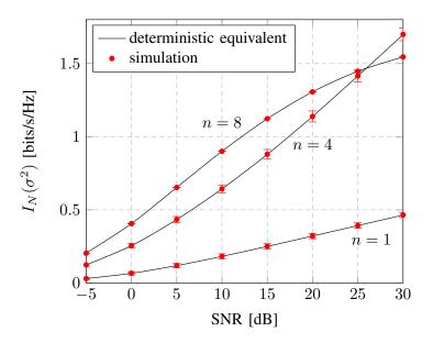
Figure 3.21: Mutual information  $I_N(\sigma^2)$  versus SNR for different numbers of transmit signatures  $n, N = 16, N_i = 8, \mathbf{P}_i = \mathbf{I}_n, \alpha = 0.5$ . Error bars represent one standard deviation on each side.
