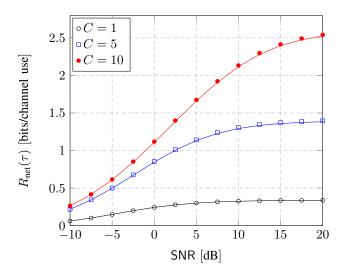
Figure 3.3: Net ergodic achievable rate  $R_{\rm net}(\tau)$  vs SNR for  $\tau=40$  and T=1000. The markers are obtained by simulations, the solid lines correspond to the deterministic equivalent  $\overline{R}_{\rm net}(\tau)$ .
