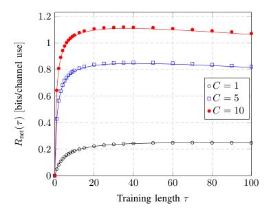
Figure 3.4: Net ergodic achievable rate  $R_{\rm net}(\tau)$  vs training length  $\tau$  for SNR = 0 dB and T=1000. The markers are obtained by simulations, the solid lines correspond to the deterministic equivalent  $\overline{R}_{\rm net}(\tau)$ .
