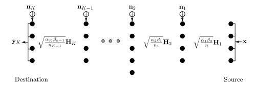
Figure 3.18: Multi-hop amplify-and-forward MIMO relay channel.
