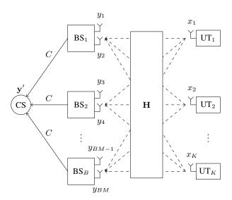
Figure 3.1: Schematic system model for M=2 antennas per BS. The BSs compress and forward their received signals to the CS via orthogonal backhaul links of capacity C bits/channel use. The CS jointly processes the received data from all BSs.
