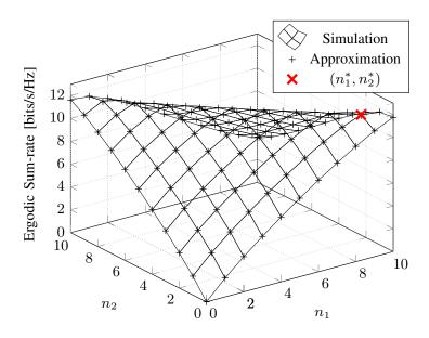
Figure 3.27: Sum-rate versus number of transmitted data-streams  $(n_1, n_2)$  for SNR = 40 dB and all other parameters as provided in Table 3.2. Solid lines correspond to simulation results, markers to the deterministic approximation by Theorem 23 (ii). As co-channel interference is dominant there is a clear gain of limiting the number of transmitted streams.
