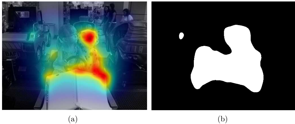
Figure 7.6: (a) shows the map of salient regions according to GBVS. (b) shows in white the area where high-saliency forbids the distractor insertion.
