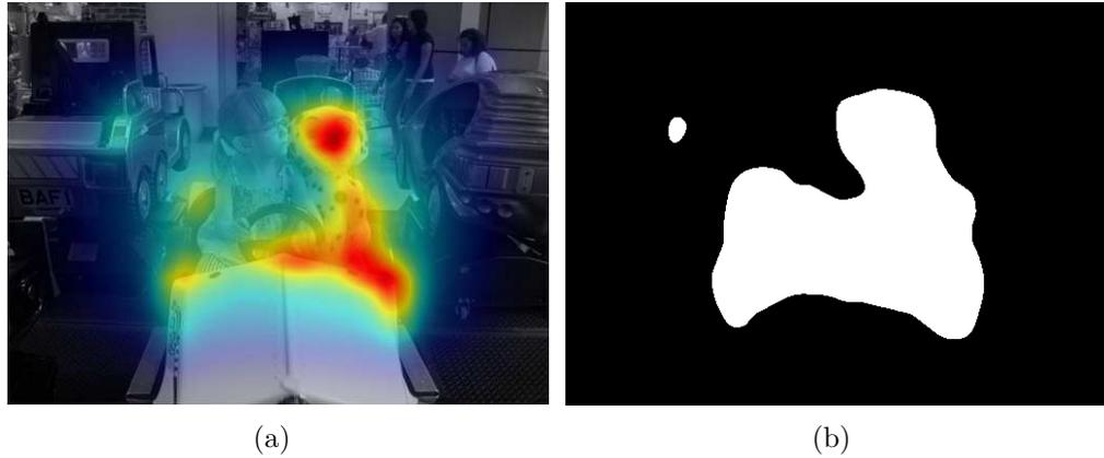
Figure 7.6: (a) shows the map of salient regions according to GBVS. (b) shows in white the area where high-saliency forbids the distractor insertion.
