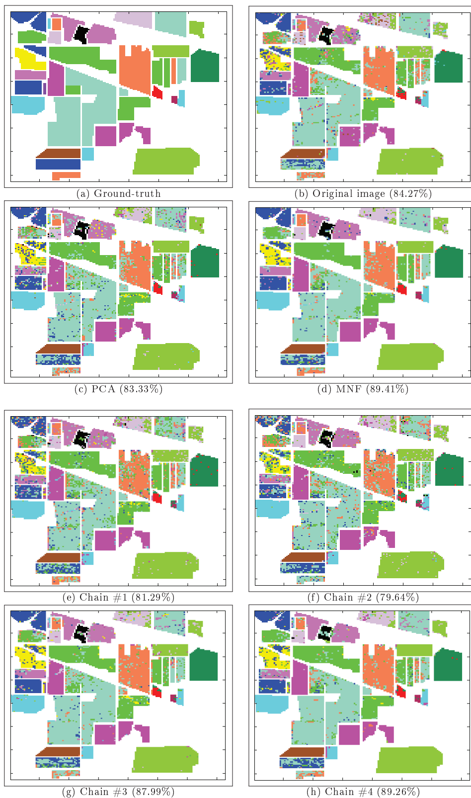
Figure 4.7: Best classification results for AVIRIS Indian Pines (using SVM classifier with Gaussian kernel, trained with 10% of the available samples per class).
