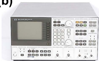
Figure 3.8 Noise measurement system: (a) a pre-amplifier (SR570, Stanford Research System) and (b) a dynamic signal analyzer (HP3562, Agilent).
