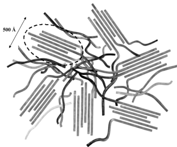
Figure 1.9: Schematic view of correlated polymeric aggregates domains [65]
