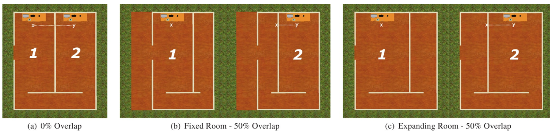
Figure 1.21 – Impossible Spaces: the virtual rooms overlaps on the real workspace [Suma 12].
