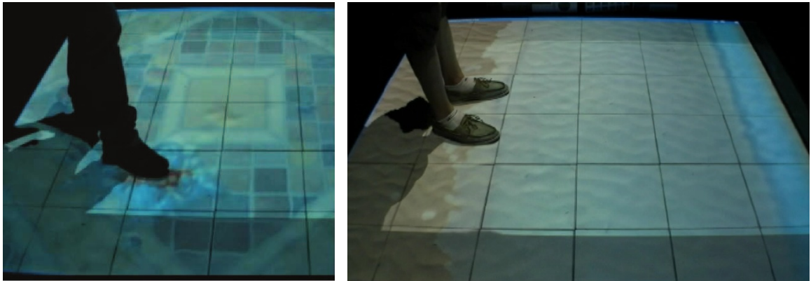
Figure 1.33 – Multimodal simulation of walking in water: visual, audio and vibrotactile feedbacks. Scenarios: a shallow water pool (a) and a wave rushing on a beach (b) [Cirio 12a].
