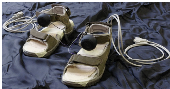
Figure 1.22 – Shoe-based device for vibrotactile feedback [Papetti 10].
