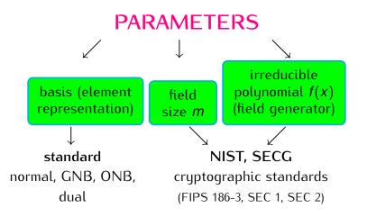
GNB, ONB - Gaussian/Optimal Normal Basis, NIST - National Institute of Standards and Technology, SECG - Standards for Efficient Cryptography Group  $\langle \Xi \rangle \langle \Xi \rangle \langle \Xi \rangle \langle \Xi \rangle$
