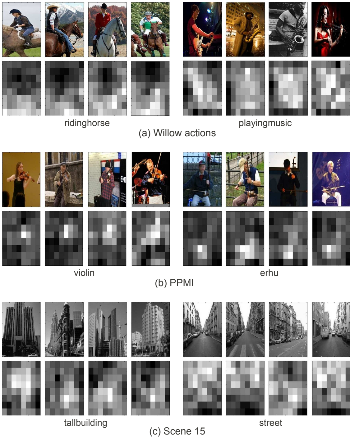
Figure 3.8: Example images and their saliency maps ( 8 \times 8 resolution) for images from two classes for each of the three databases (higher values are brighter). Notice how the maps adapt to the content of the image and highlight the spatially salient regions per image.
