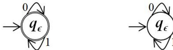
Figure 3.5: Initial DFAs M_1^1 and M_1^0 for \Sigma = \{0, 1\} . State q_\epsilon is accepting in M_1^1 and non-accepting in M_1^0 .
