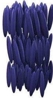
Figure 6.4: Sketch of the structure of a smectic (more precisely, smectic A) liquid crystal. Illustration reproduced from Wikimedia Commons.
