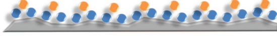
Fig. 1 In order to smooth the potential and obtain a two-dimensional homogeneous Fermi liquid, {}^3\text{He} is adsorbed on a graphite substrate preplated with a solid {}^4\text{He} layer.
