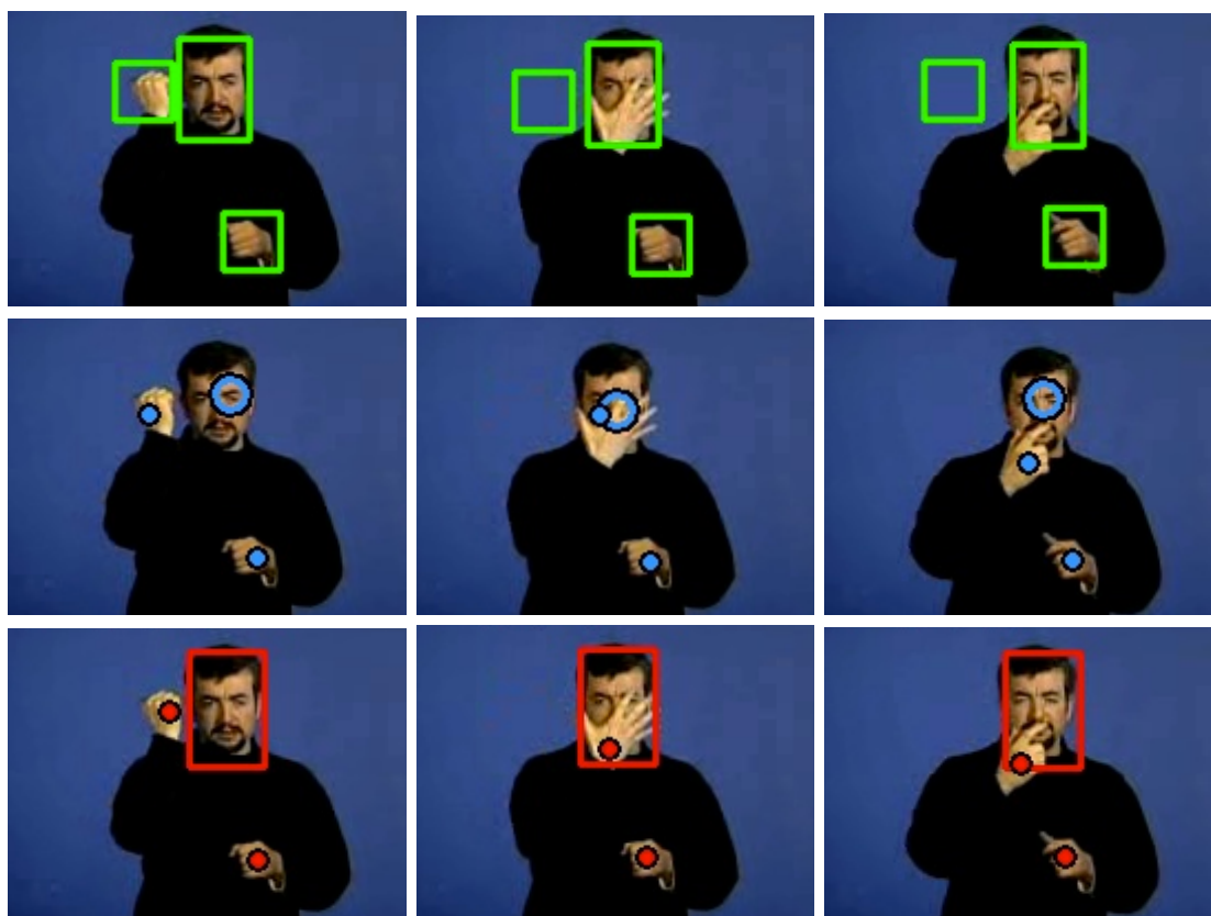
Figure 4.18: Tracking results. For Lefebvre (top row), Gianni et al. (middle row) and the proposed approach (bottom row).
