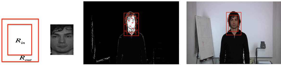
Figure 4.11: (a) Illustrates the proposed face model. (b) shows the rectangular model lying over the skin probability map when \rho_{R_T} is maximal and (c) represents the best matching position for the template registration.
