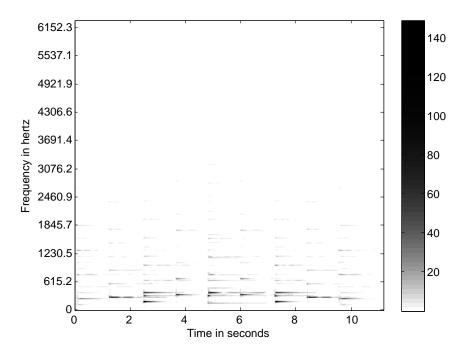
Figure 5.3.: Spectrogram of the piano excerpt. The excerpt is composed of the notes C-D-E-F-G-F-E-D-C played successively on the right hand, while the left hand plays the notes C-G-E-G-C at half the speed.
