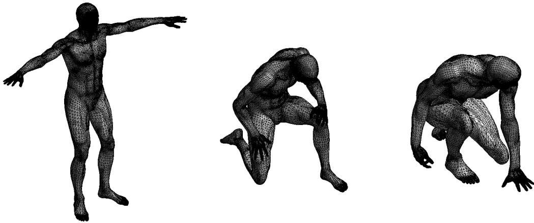
(a) High-resolution Delaunay triangulation of closed (compact and without boundaries) surfaces
