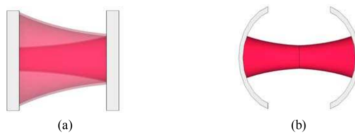
Fig. 5.1 Illustration of Gaussian beams properties in FP cavity (a) expansion of the spot size after single reflection by planar mirror (b) confinement of the beam after multiple reflections by curved mirrors, whose radii of curvature fits with the beam radius of curvature at the specific mirror locations.
