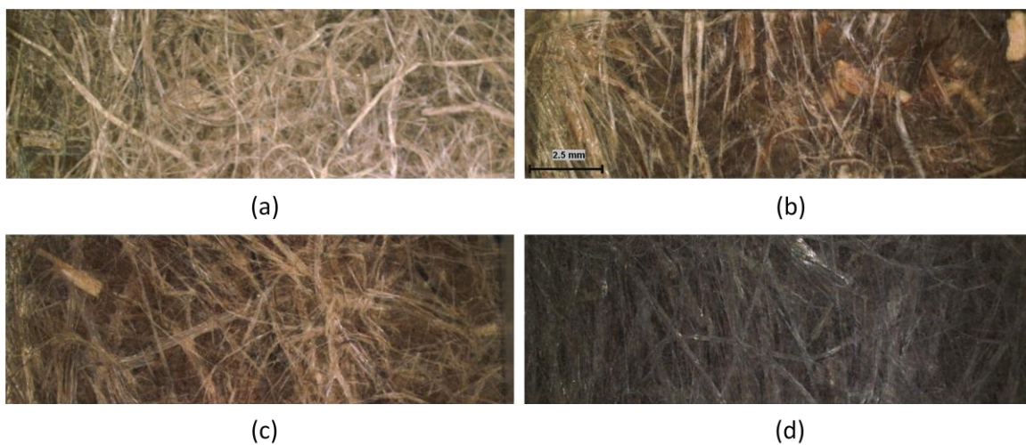
Figure VI.4. Optical micrographs of aged NDF/PP composite surfaces : (a) aged in distillate water (23°C), (b), (c), (d) aged at 23°C, 70°C and 90°C respectively and at 80% HR during three months
