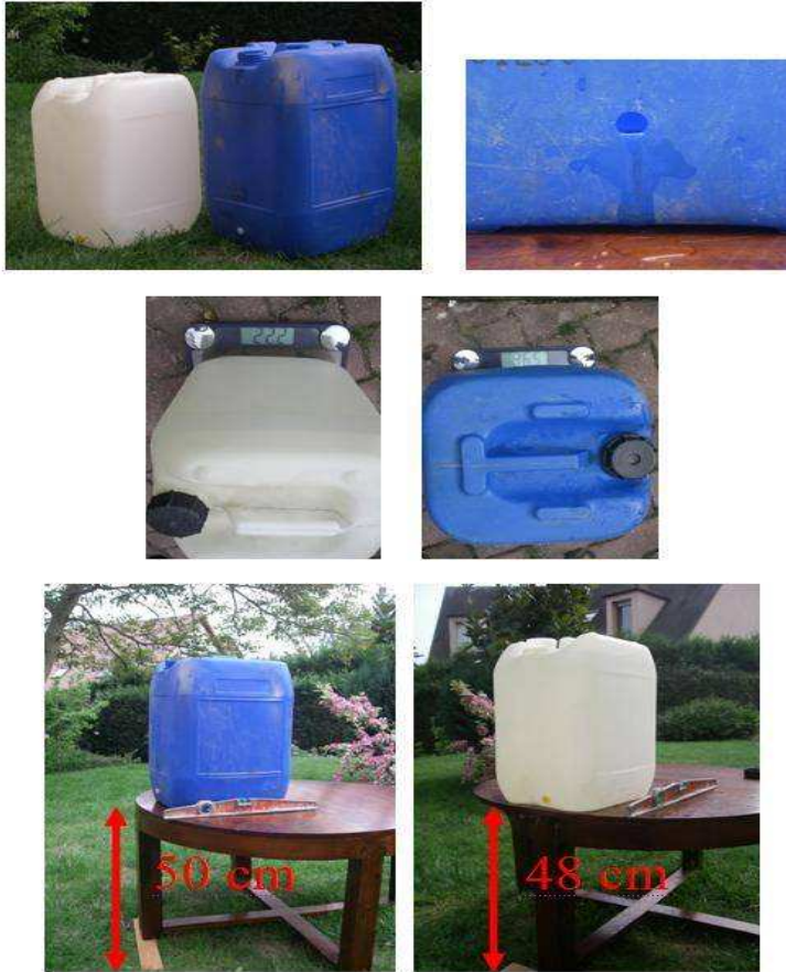
FIG. 8.1 – Example of atypical experiments in fluid mechanics : emptying jerry cans, preparation of experiments.
