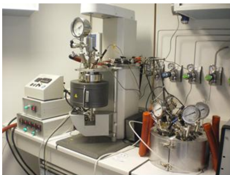
Executive Abstract Figure 2: Experimental set-up for hydrogen gas reactivity experiments on clay materials with a one liter titanium reactor (on the left) and four stainless steel reactors of 300 mL (on the right). The whole system is connected on line with a gas chromatograph through an automated system of valves.
