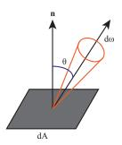
Figure III.1: The geometry of radiance.
