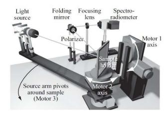
Figure III.10: Gonio-reflectometer for isotropic BRDF measurement. (From [Li 2005])
