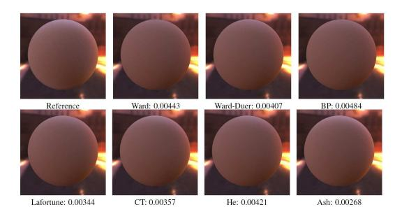
Figure III.22: Comparison between several analytical models for *beige-fabric* from MERL-MIT database — figures from left to right: reference, Ward, Ward-Dür, Blinn-Phong, Lafortune, Cook-Torrance, He, and Ashikhmin-Shirely. The numbers below each figure represent the  $L^2$  metric error value. (From [Ngan 2005] supplemental material)
