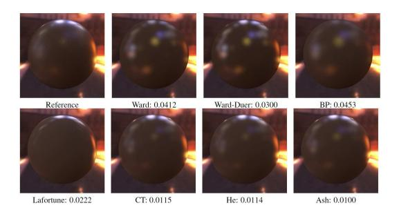
Figure III.23: Comparison between several analytical models for *fruitwood-241* from MERL-MIT database — figures from left to right: reference, Ward, Ward-Dür, Blinn-Phong, Lafortune, Cook-Torrance, He, and Ashikhmin-Shirely. The numbers below each figure represent the  $L^2$  metric error value. (From [Ngan 2005] supplemental material)
