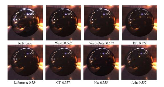
Figure III.24: Comparison between several analytical models for *chrome* from MERL-MIT database — figures from left to right: reference, Ward, Ward-Dür, Blinn-Phong, Lafortune, Cook-Torrance, He, and Ashikhmin-Shirely. The numbers below each figure represent the  $L^2$  metric error value. (From [Ngan 2005] supplemental material)
