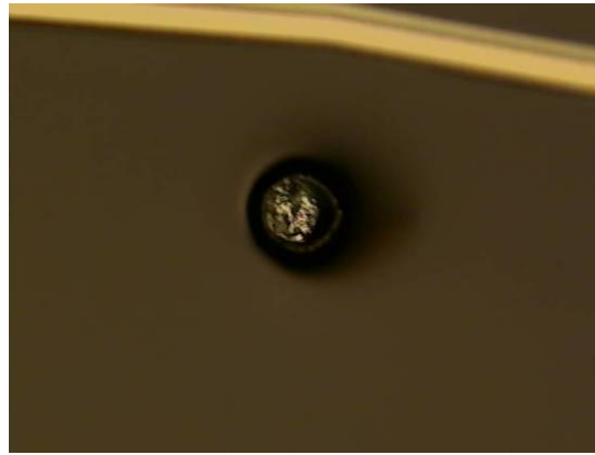
FIGURE 1.25 – Picture of a micropipe taken on-wafer during the fabrication process of SiC diodes at CNM of barcelona
