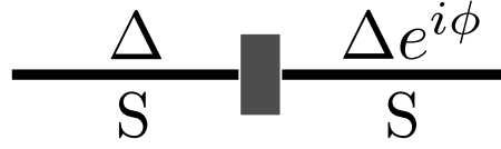
Fig. 5.5: Schematic picture of a Josephson junction. Without loss of generality, one can consider that the superconducting parameter has equal absolute value in the two superconductors. The left superconductor is conventionally considered real, while there is a superconducting phase \phi in the right wire. In the middle there is an insulating barrier or a metallic region.
