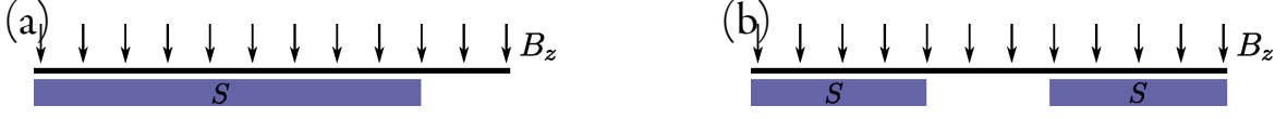
Fig. 5.1: Schematic representations of (a) superconductor-normal and (b) superconductor-normal-superconductor junctions. They are created by having the spin-orbit coupled semiconducting wire added on top of an s -wave superconductor ( S ). A perpendicular magnetic field B_z acts on the wire.
