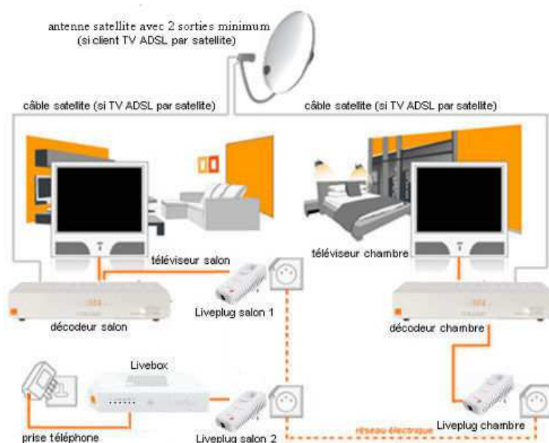
Figure 5.1: Possible configuration of the Orange multiscreen TV offer using 3 Orange Liveplugs (Picture downloaded from the Orange online support website).
